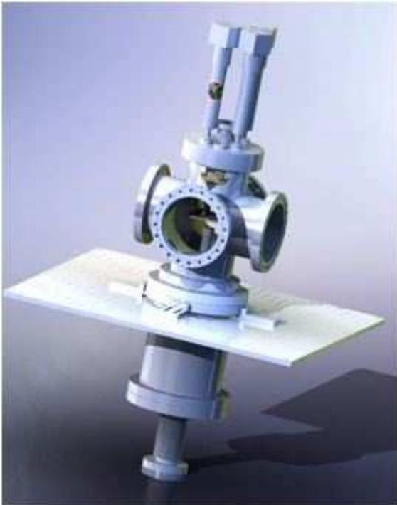
Figure 4: Diamond Field Emitter Cathode test stand
