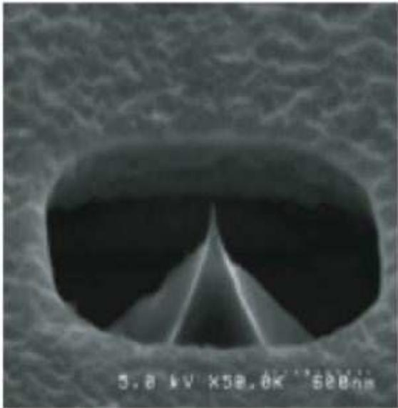
Figure 5: Single Diamond Field Emitter example
