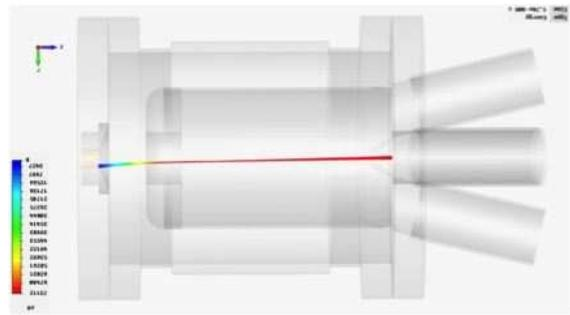
Figure 6: Photoelectric cathode test stand schematic
