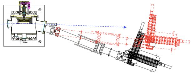
Figure 2: Top view of the energy spectrometer. The beam is coming from the left (dashed line) and impinges at  $2.5^\circ$  on the grating. The ES can be moved to track the focal line (see text): solid and dashed images. The 0-order radiation continues to the beamlines.
