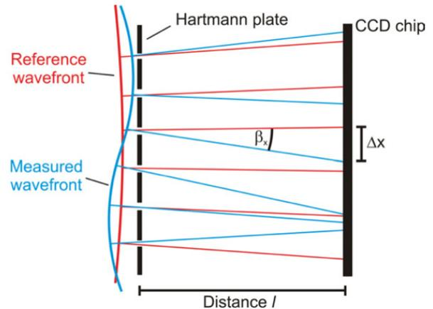
Figure 3: The incoming beam is divided into an array of beams by the Hartmann plate. The centroid deviation  $\Delta x$  from a known reference spot position divided by the distance  $l$  yields the local wavefront gradient  $\beta_x$  relative to the reference wavefront (from [20]).
