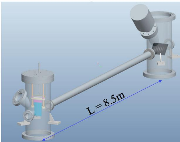
Figure 4: Section of a FERMI@Elettra branchline dedicated to spatial coherence measurements.
