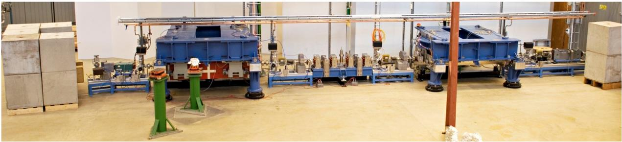
Figure 2: The two undulators ( U48, the modulator, right and UE56, the elliptical radiator, left) in the MAX-lab test FEL.
