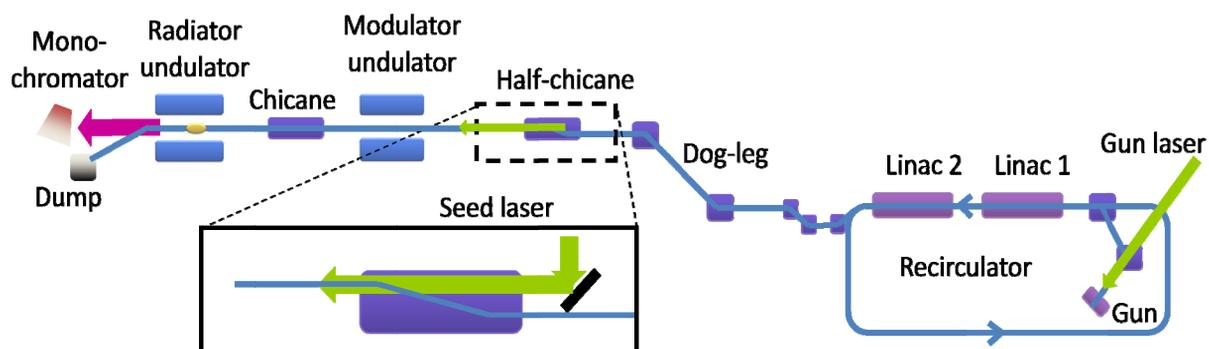
Figure 1: Layout of the MAX-lab test FEL.
