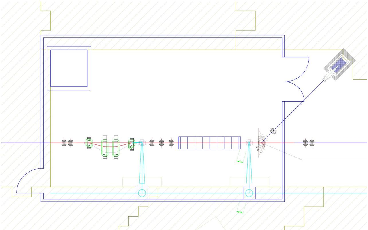
Figure 1: Preliminary drawing of the beamlines of the THz facility showing the magnetic chicane for bunch compression and the wiggler along with the necessary focussing quadrupoles and deflecting dipoles. The outline of the THz laboratory on the rooftop of the accelerator vault is shown in dark blue. The projected optical beam transport path is sketched in cyan.
