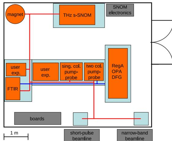
Figure 5: Projected layout of the THz optical laboratory.
