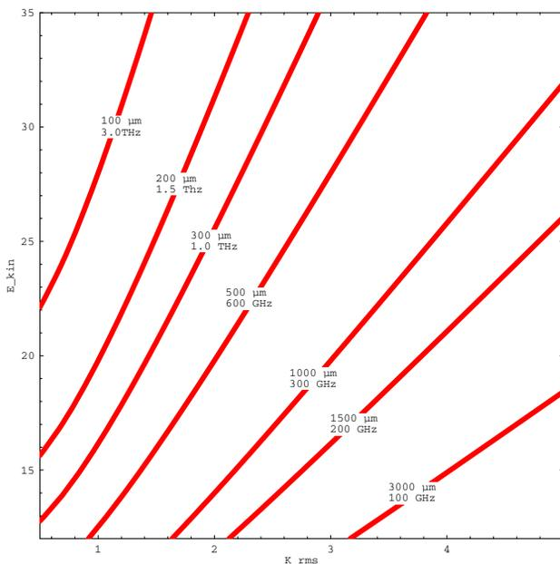
Figure 3: Tuning range of a 30 cm period length wiggler at ELBE beam energies.
