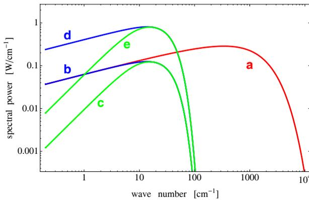
Figure 2: Spectral power density of coherent synchrotron radiation from a 40 MeV electron beam in a  $\rho=1$  m bending dipole into a  $(60 \text{ mrad})^2$  acceptance angle – **a** from a point charge with  $Q=77$  pC at 13 MHz repetition rate, **b** and **c** from bunches of 150 fs (r.m.s.) bunch length with 77 pC, **d** and **e** from 1 nC bunches with 500 kHz repetition rate. Curves **c** and **e** include diffraction losses due to the limited source size in a 40 mm high vacuum chamber.
