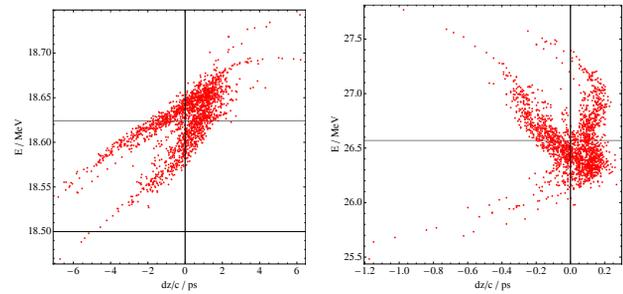
Figure 4: Longitudinal phase space of the electron beam after the first linac (left) and after bunch compression (right). Note the different energy spread and time scales.
