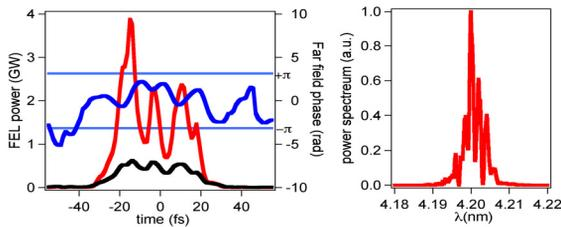
Figure 6: (a) FEL 4.2-nm fundamental power at the undulator exit (red) and on-axis far field intensity (black) predicted by GINGER S2E simulations. The blue line plots the on-axis far field eikonal phase. (b) Far field power spectrum of the FEL radiation as predicted by S2E simulations.
