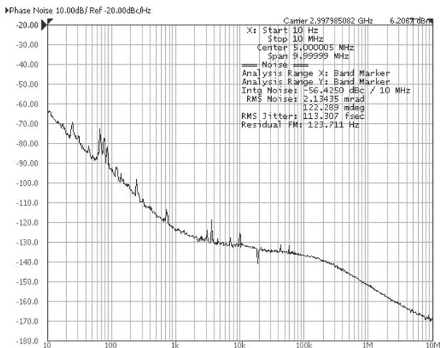
Figure 5: Measured RMS jitter of the Rx-output signal is 113.3 fs, integrated from 10 Hz to 10 MHz.
