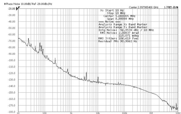
Figure 4: Measured RMS jitter of the reference signal is 106.6 fs, integrated from 10 Hz to 10 MHz.
