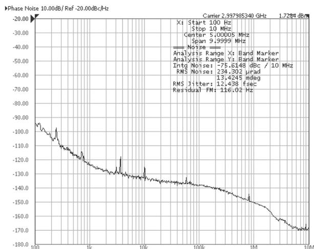
Figure 6: Measured RMS jitter of the reference signal is 12.4 fs, integrated from 100 Hz to 10 MHz.
