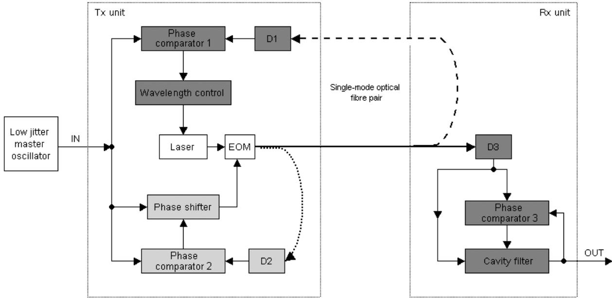
Figure 1: Block diagram of the Electro-optical synchronization system.
