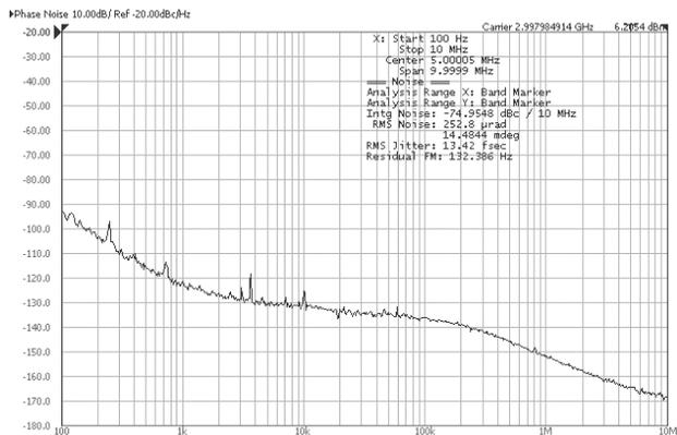
Figure 7: Measured RMS jitter of the Rx-output signal is 13.4 fs, integrated from 100 Hz to 10 MHz.
