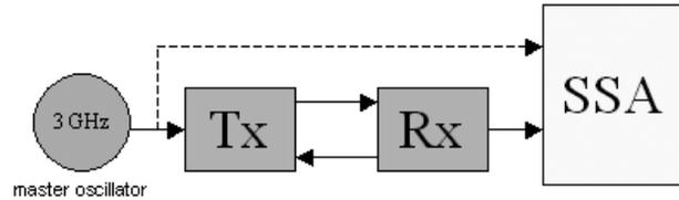
Figure 3: RMS jitter measurement diagram.
