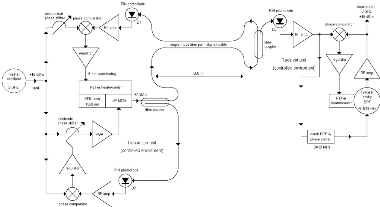
Figure 2: Detailed block diagram of the electro-optical synchronization system.
