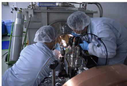
Figure 2: Scene in the replacement of the gun cathode.
