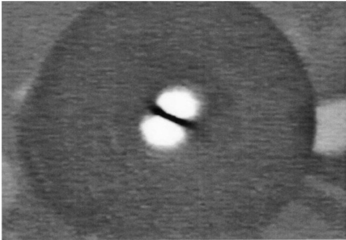
FIG. 4. Infrared impinging on the optical beam dump showing the second harmonic TEM 01 mode. The image is tilted due to relative misalignments in the system with perhaps additional contributions from coupling due to misalignment in our optical collimator.
