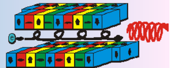
4. mode: linear polarization under various angle shift of magnetic rows antiparallel
