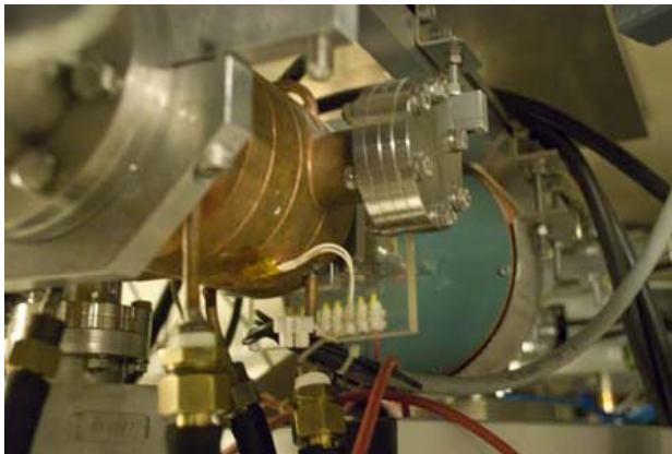
RF gun \approx 1.8 MeV Thermionic ++
