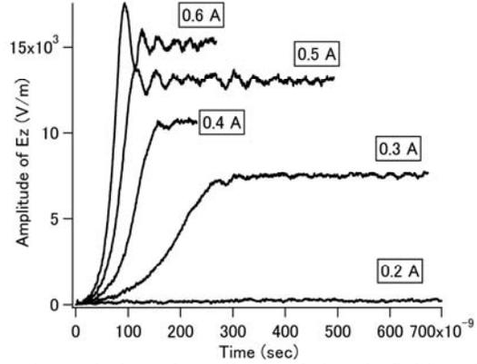
Figure 3: Evolution of amplitude of electric field  $E_z$  for sidewall grating for various beam currents.
