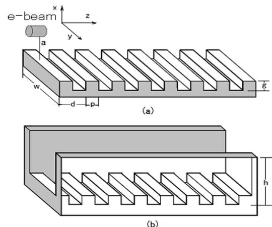
Figure 1: Schematic of grating model. (a) general grating (b) sidewall grating
