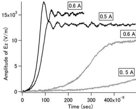
Fig. 2 Evolution of amplitude of electric field  $E_z$  (gray curves for general grating and black curves for sidewall grating).
