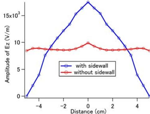
Figure 4: Transverse profile of  $E_z$ .
