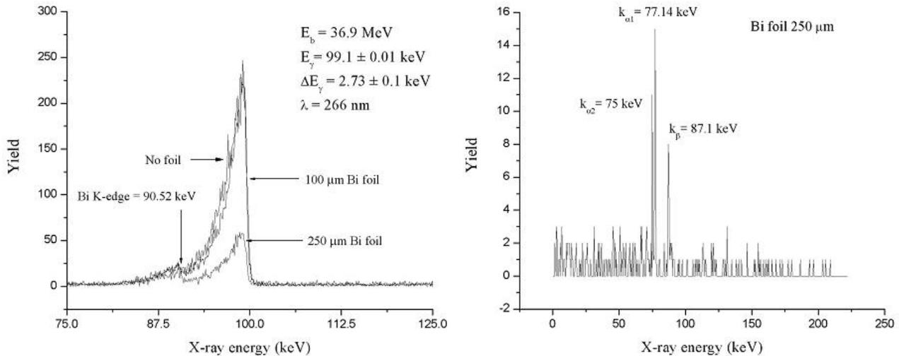
Figure 3: (a) Transmitted LCS spectra through Bi foils of different thicknesses. The pile up peaks (not shown) vanish when a 250  $\mu\text{m}$  thick foil is used. (b) LCS-induced x-ray fluorescence from a 250  $\mu\text{m}$  thick Bi foil, the brightest line is the  $k_{\alpha 1}$  and is located at 77.14 keV. In these experiments lead was present in the shielding.
