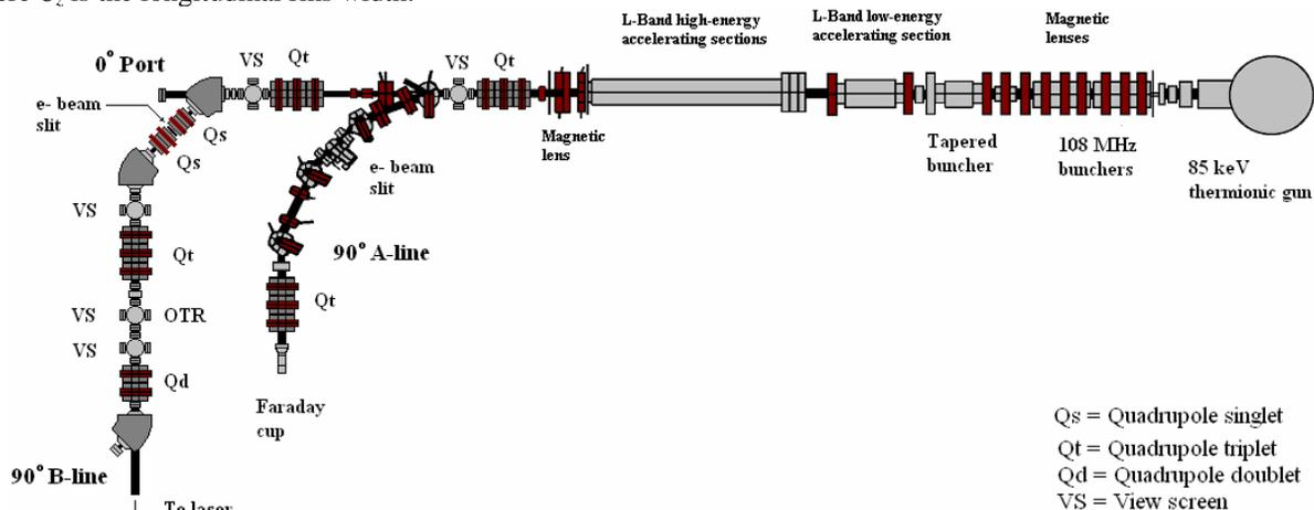
Figure 1: IAC LINAC layout. The B-line is a dedicated to LCS experiments.
