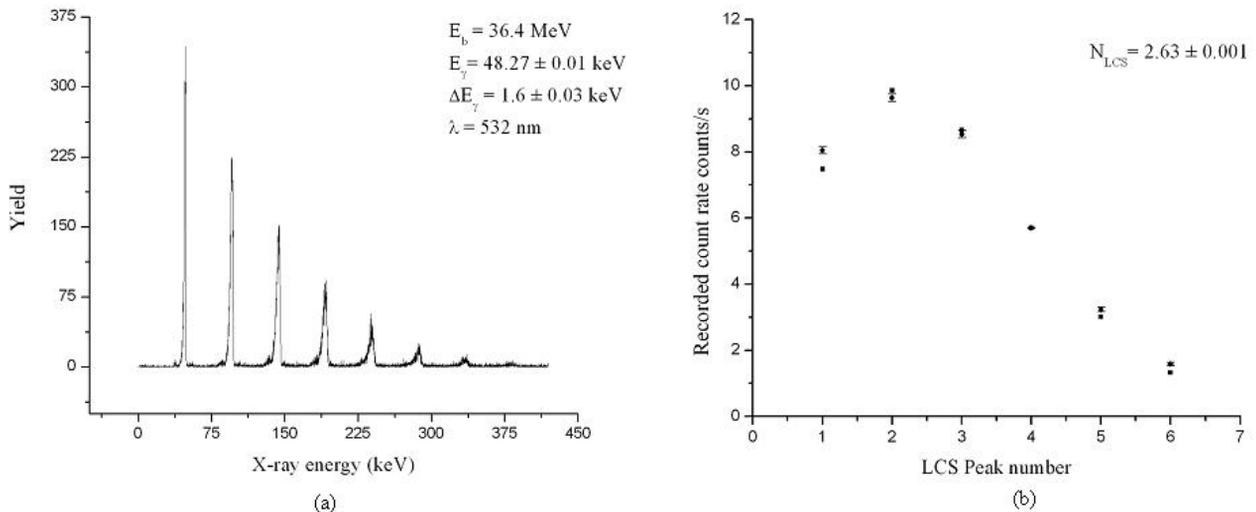
Figure 2: (a) LCS spectrum resulting from the interaction of a 36.4 MeV electron beam with 532 nm laser photons. (b) Average number of LCS photons per collision reaching the germanium detector. The x-ray yield was found to be equal to 0.005 photons/e-Sr. The square points correspond the count rates in each LCS peak for  $N_{LCS} = 2.63$ .
