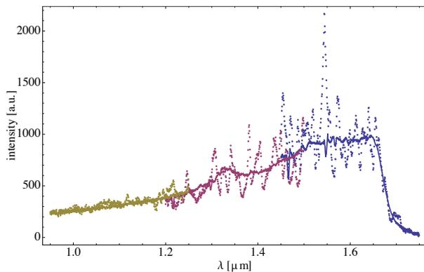
Figure 7: Single shot (dots) and averaged (line) CTR spectrum between  $0.95 \mu\text{m}$  and  $1.7 \mu\text{m}$  measured with a commercial InGaAs spectrograph. The response of the detector is basically flat between  $1.0 \mu\text{m}$  and  $1.7 \mu\text{m}$ .
