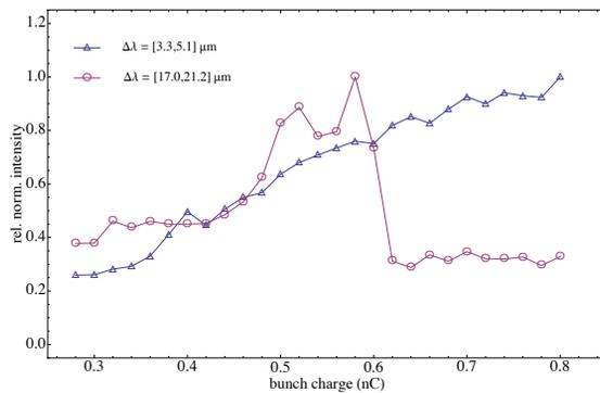
Figure 4: Normalized spectral intensity for two wavelength bands as function of the bunch charge. The band  $3.3 - 5.1\ \mu\text{m}$  is dominated by microstructures while the band  $17 - 21\ \mu\text{m}$  results predominantly from the leading current spike of the compressed bunches.
