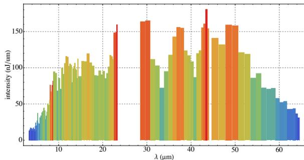
Figure 2: Intensity of coherent transition radiation from electron bunches with  $0.8\ \text{nC}$  charge for normal FEL-mode operation. The spectrum was recorded with 6 different grating stages and averaged over 300 shots.
