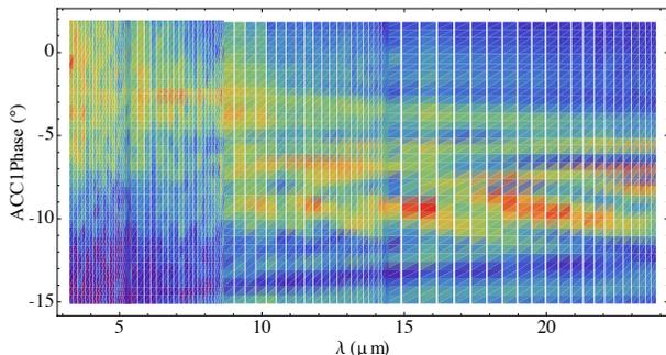
Figure 3: Normalized spectral intensity for  $3\ \mu\text{m} < \lambda < 24\ \mu\text{m}$  as function of the off-crest phase of the first acceleration module. Each wavelength bin is normalized to its maximum value individually. A typical FEL operation point is at  $-4^\circ$  to  $-6^\circ$  off-crest.
