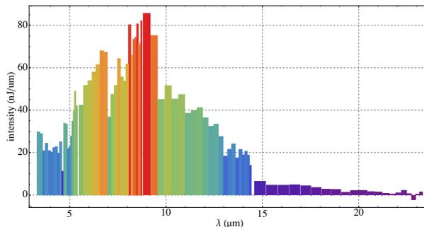
Figure 5: Intensity of coherent transition radiation from electron bunches with  $0.8\ \text{nC}$  charge for both bunch compressors set to on-crest operation.
