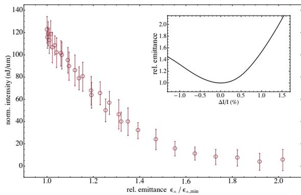
Figure 9: Intensity of coherent transition radiation for  $6.2 < \lambda < 8.6 \mu\text{m}$  as function of the expected beam emittance. The emittance as function of the solenoid current was determined by ASTRA simulations [8] as shown in the plot inset.
