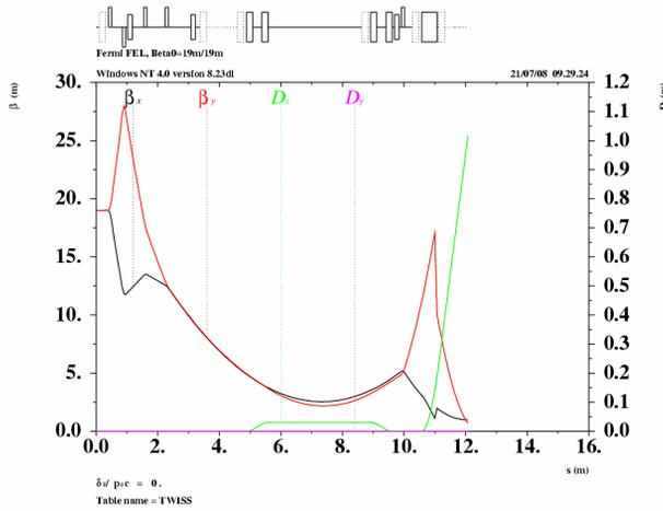
Figure 6: Optics of the laser heater spectrometer line.
