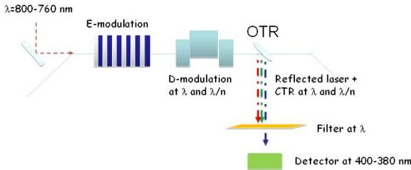
Figure 3: Layout of the energy modulation monitor system.
