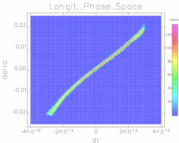
Figure 7: longitudinal phase space of the electron beam after BC1 (compressed beam).
