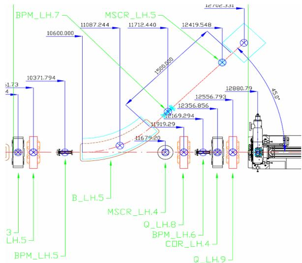
Figure 5: Layout of the laser heater spectrometer line.
