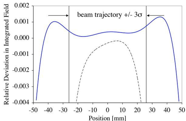
Figure 6: The solid(dashed) curve shows bench measurements of BX12 after(before) final modification and shimming.
