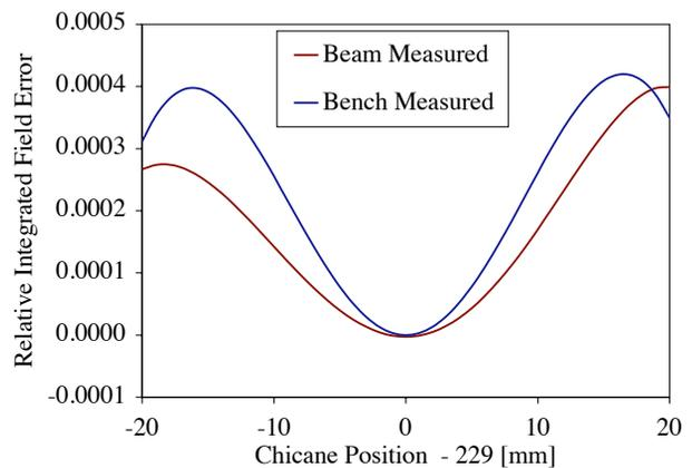
Figure 2: High resolution beam measurements of relative integrated field error compared with the sum of the bench measurements for both inner dipoles with the nonlinear components subtracted off of both.
