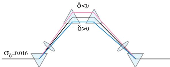
Figure 1: Schematic of a bunch compressor.
