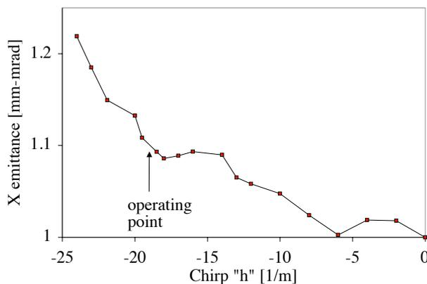
Figure 4: Based on tracking, the calculated normalized emittance after BC1 is plotted as a function of the chirp parameter for an initial emittance of  $1.0\ \mu\text{m}$ .
