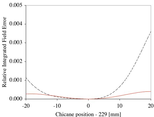
Figure 3: Chicane scan measurements of the net inner dipoles before (solid curve) and after (dashed curve) modifications to the original dipole.
