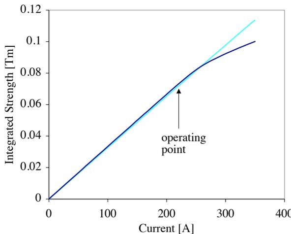
Figure 5: Integrated strength as a function of main coil current for the unmodified (light blue) and modified (dark blue) BX12 magnet.
