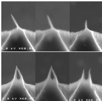
Figure 10. Examples of self-healing behavior of nanotips.
