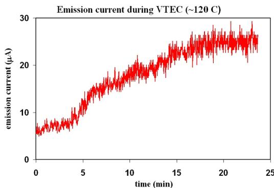
Figure 5. Typical emission current data during a low temperature VTEC treatment.
