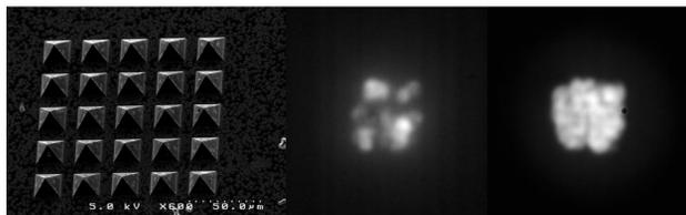
Figure 4. Electron beam from a 5x5 diamond FEA before and after VTEC.
