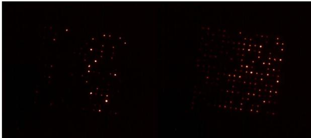
Figure 3. (left) Before VTEC  $\sim 30\%$  of tips active, (right) after VTEC  $\sim 60\%$  of tips active.
