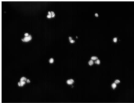
Figure 2. Beamlets from individual adsorbates on diamond nanotips (centroid spacing  $\sim 300\mu\text{m}$ ).
