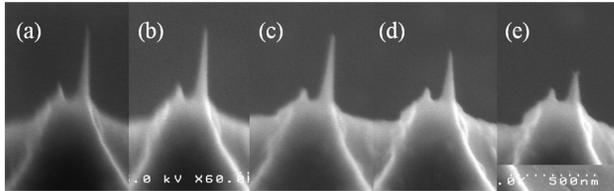
Figure 9. Evaporation progression of a single nanotip.
