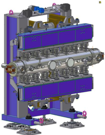
Figure 1: Schematic drawing of the USAXS IVU.
