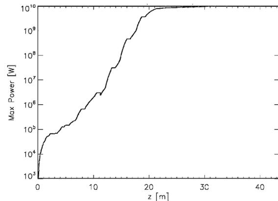
Figure 8. Evolution of peak FEL power along the undulator for SPARX 10 pC case.
