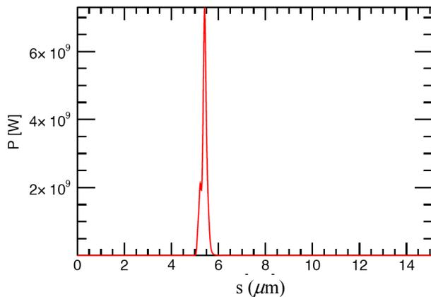
Figure 9. Peak FEL power as a function of  $s$  at saturation, SPARX 10 pC case.
