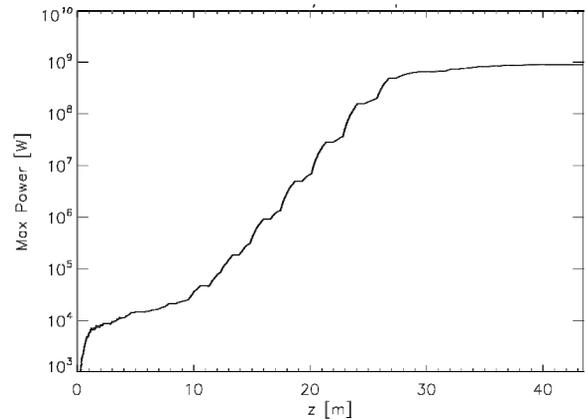
Figure 3. Evolution of peak FEL power along the undulator for SPARX 1 pC case.
