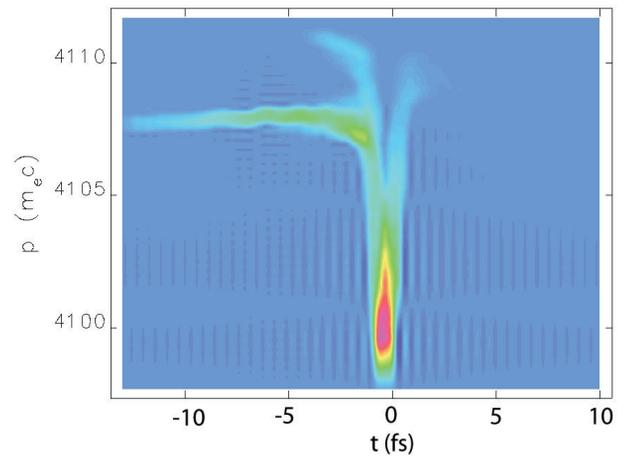
Figure 6. Longitudinal phase space at undulator entrance for SPARX 10 pC case.
