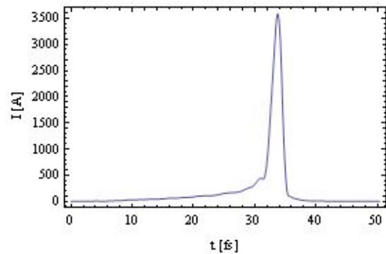
Figure 7. Current profile in SPARX 10 pC case.
