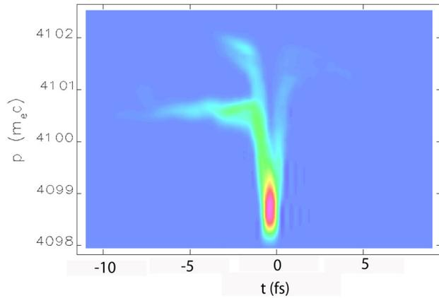
Figure 1. Longitudinal phase space at undulator entrance for SPARX 1 pC case.
