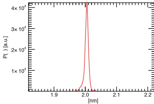
Figure 5. Saturation spectrum, SPARX at 1 pC.
