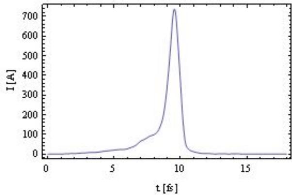
Figure 2. Current profile in SPARX 1 pC case.
