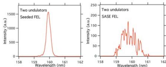
Figure 7: Spectra of the seeded FEL and SASE with small FEL gain after the second undulator, left: seeded FEL, right: SASE.
