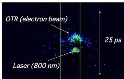
Figure 4: Longitudinal position of the 800 nm laser and the electron bunch measured with a streak camera. Two pulses are intentionally displaced in the figure.
