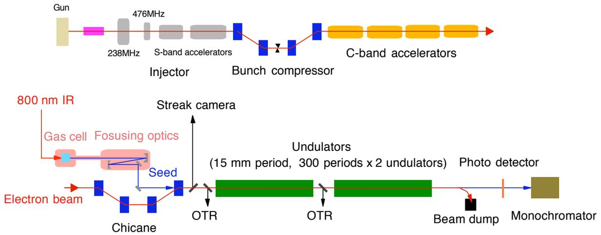
Figure 1: Schematic of the SCSS test accelerator.
