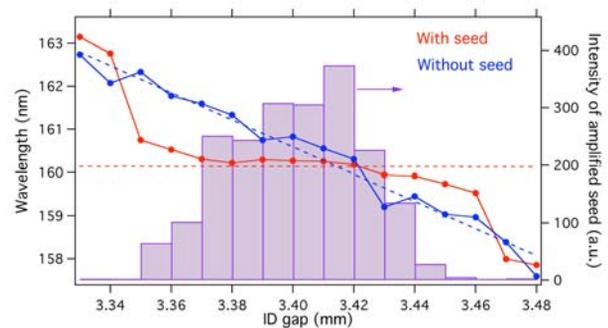
Figure 8: Central wavelengths of the seeded FEL (line-points in red) and SASE (line-points in blue) as a function of the undulator gap. Black dashed line is the wavelength of the seed. Bars show the intensity of the seeded FEL. The electron bunch length is 4 ps and only the first undulator gap is closed
