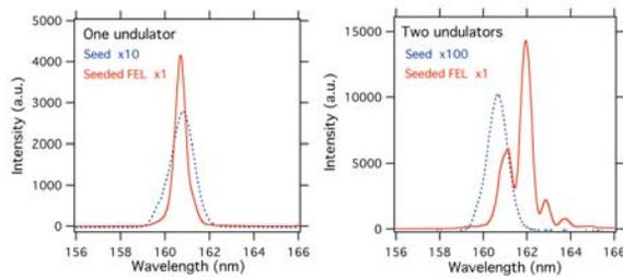
Figure 5: Spectra of the seeded FEL with large FEL gain, left: after the first undulator, right: after the second undulator. Lines in red are the spectra of the seeded FEL and blue dotted lines are those of the seed.
