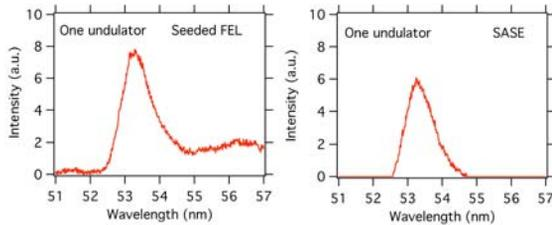
Figure 9: Spectra of 3rd harmonics of the seeded FEL and SASE after the first undulator, left: seeded FEL, right: SASE. The electron bunch length is 4 ps and the spectra are mainly spontaneous emission. The intensity increase at the long wavelengths in the spectrum of the seeded FEL is due to stray light of 800 nm laser.
