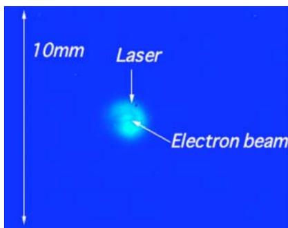
Figure 3: Transverse overlap between the 800 nm laser and the electron beam observed on the OTR screen.
