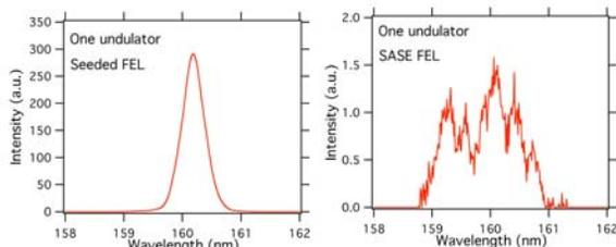
Figure 6: Spectra of the seeded FEL and SASE with small FEL gain after the first undulator, left: seeded FEL, right: SASE.
