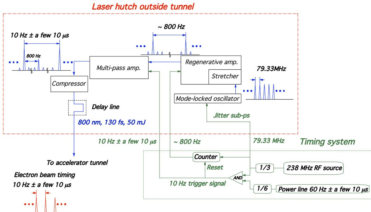
Figure 2: Synchronization system of the titanium-sapphire laser to the electron beam.
