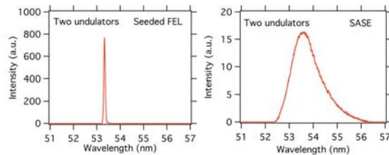
Figure 10: Spectra of 3rd harmonics of the seeded FEL and SASE after the second undulator, left: seeded FEL, right: SASE. The electron bunch length is 4 ps and the SASE spectrum is mainly spontaneous emission.
