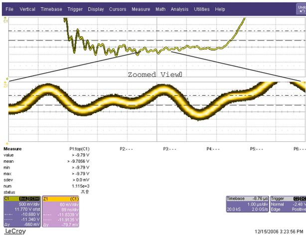
Figure 4: Klystron voltage stability of the inverter type modulator. The upper figure: klystron beam voltage, lower figure: zoomed view.
