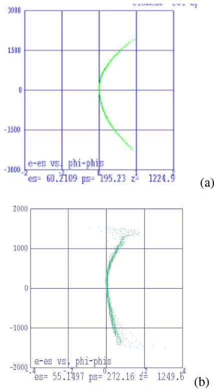
Figure 2: Bunch shape after Chicane-2 in case of RF-gun energy of 3 MeV (a) and 5 MeV (b).  $es$  represents the synchronous particle energy,  $phis$  the synchronous particle phase. The vertical axis is  $e - es$  in MeV and the horizontal axis is  $phi - phis$  in degrees. One degree corresponds to about 1 ps.
