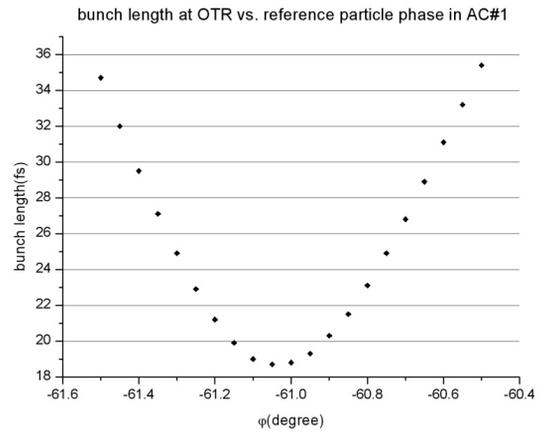
Figure 3: Bunch length's dependence on AC1 RF phase
