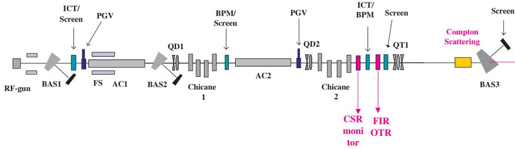
Figure 1: Layout of Linac. (QD: quadrupole doublet, ICT: integrated current transformer, FS: focusing solenoid, AC: accelerating column, QT: quadrupole triplet, OTR: optical transition radiation, BAS: beam energy analyzer, and YAG: YAG screen).
