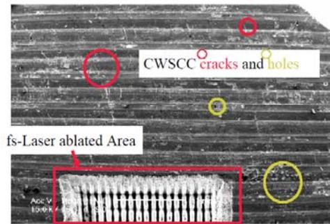
Figure 8: A large number of typical cold worked stress-corrosion cracking(CWSCC) cracks and holes are found in the 316L stainless-steel sample surface which have often been used in the boiling light water reactor (BWR) shroud and other reactor internal components after the JIS(Japan Industry Standard) defined  $MgCl_2$  SCC test of 20 hours.
