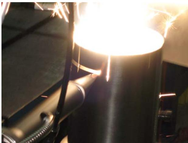
Figure 3a: A Fugen Zirconium alloy pressurized tube of about 4.3mm thick and 117.8mm inner diameter was successfully and quickly cut with 6m per a minute using 20 bar compressed and focused N<sub>2</sub> gas flow and IPG 5kW fiber laser.
