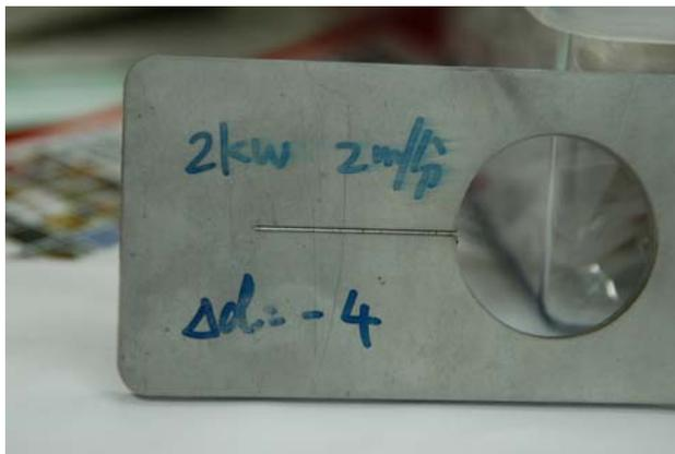
Figure 2: A Stainless-steel plate of 4mm thick and 40mm wide and 80mm long was successfully and quickly cut using 20 bar compressed and focused N<sub>2</sub> gas flow and IPG made 2 kW CW Ytterbium fiber laser. The 2kW fiber laser system usually has a capability of thick metal plate cutting from a few mm up to ten and several mm.
