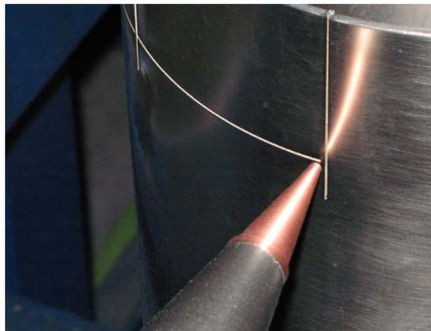
Figure 3b: The Zirconium alloy tube was cut with very high speed of 6m per a minute, and cut-width was as narrow as 0.25mm or 0.15mm. Surface condition of the cutting edges is very beautiful and very smooth and slightly narrower than the Stainless steel cases.
