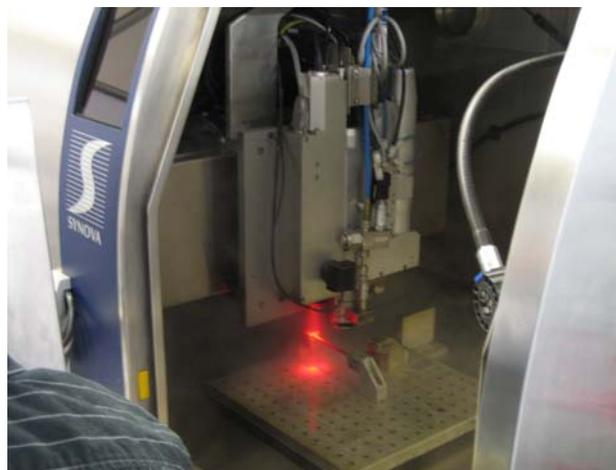
Figure 4: Water jet-guided laser named LMJ(Laser Micro-Jet ) driven by 100-200W pulsed YAG laser manufactured by Synova S.A., Switzerland is another typical example of the new, commercially-available, and advanced industrial lasers.
