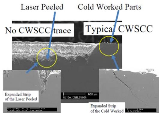
Figure 9: A cross-sectional SEM picture of the 316L stainless-steel sample after the JIS (Japan Industry Standard) defined Hot  $MgCl_2$  SCC test.
