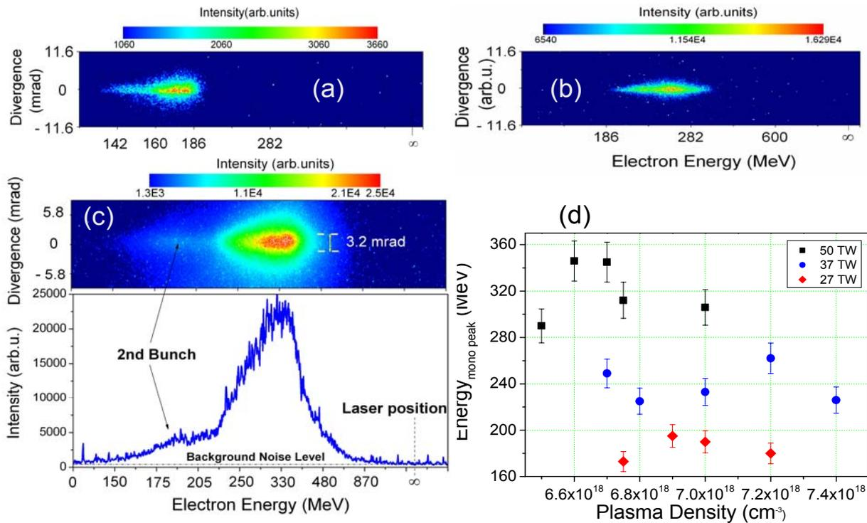
Figure 2: Quasimonoenergetic electron beams produced in 4 mm-long gas jet at various laser powers (27-50 TW) and plasma densities  $6.5 \times 10^{18} - 7.5 \times 10^{18} \text{ cm}^{-3}$ .
