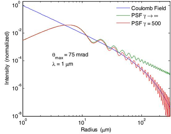
Figure 2: Point spread function of the OTR source distribution for a lens acceptance angle of 75 mrad. Shown are the Coulomb field for  $\gamma = 500$  and the PSF at the same  $\gamma$  and for  $\gamma \rightarrow \infty$ .
