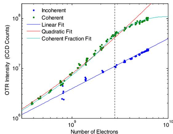
Figure 4: Dependency of OTR light intensity on the bunch charge. The data shown is for  $250 \text{ MeV}$  and uncompressed bunches. The coherent fraction fit uses the fit from Fig. 5.
