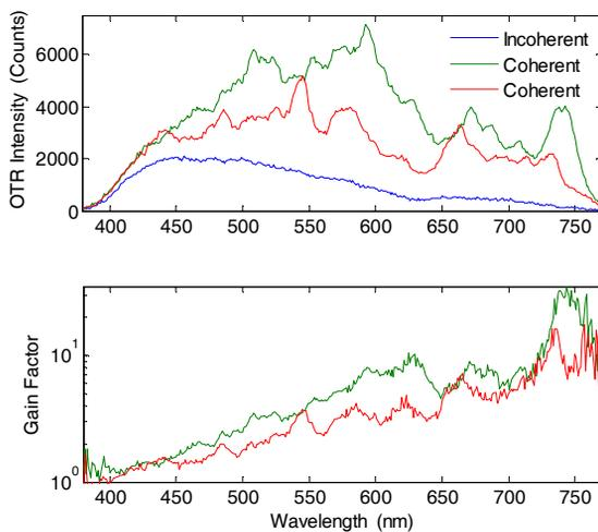
Figure 6: OTR light spectra after BC1 with the beam under normal compression (red and green) and with the coherence suppressed (blue). The spectra are in the upper panel and the spectral gain factor (ratio of coherent to incoherent spectrum) in the lower one.
