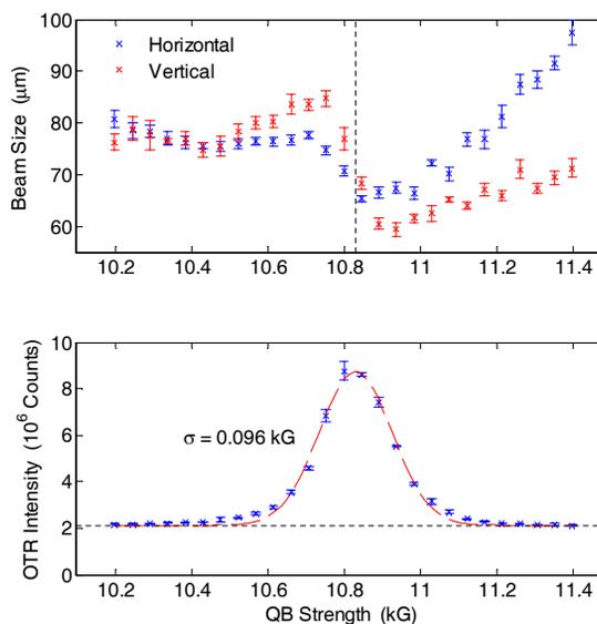
Figure 3: OTR intensity (lower) and beam sizes (upper) measured downstream of BC1 at OTR12 as a function of the dispersion correction quadrupole (QB) in the first dogleg with no bunch compression. The vertical line indicates the peak of the OTR intensity curve.
