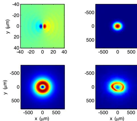
Figure 7: Simulation of COTR image. Upper panel left is the horizontal component of the source field, right is the beam distribution, lower panel left is the simulated COTR image and right the measured image.
