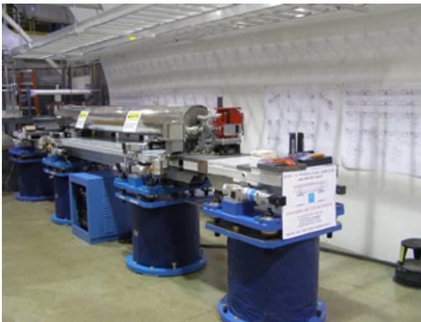
Figure 13: Long-term test stand. The single undulator system is accurately positioned with respect to a mock tunnel simulating Undulator Hall at SLAC.
