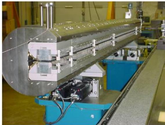
Figure 3: The prototype undulator. The magnetic structure is visible, housed in the titanium strongback.
