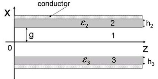
Figure 1: A double slab structure for Cherenkov free-electron laser
