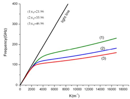
Figure 3: Dispersion curves for different relative permittivity.
