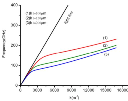
Figure 2: Dispersion curves for different slab thickness .
