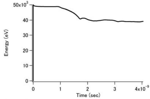
Figure 7: Average energy loss of the electron beam.
