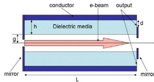
Figure 4: Simulation model of Cherenkov FEL.
