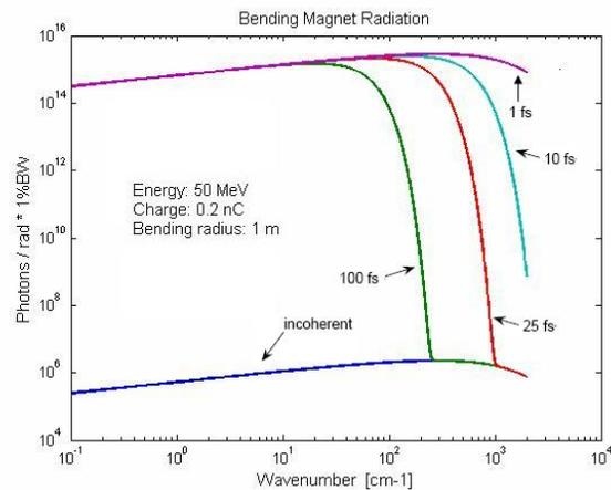
Figure 1: Synchrotron radiation from a bending magnet at different bunch lengths.
