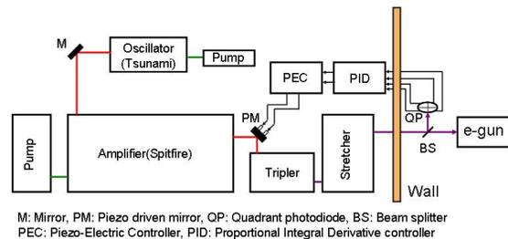
Figure 2: Beam pointing stabilization unit.
