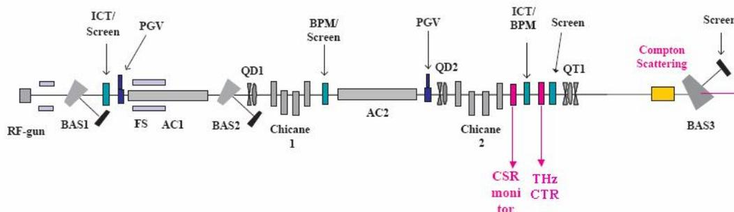
Figure 3: Layout of fs-THz Linac. (QD: quadrupole doublet, ICT: integrated current transformer, FS: focusing solenoid, AC: accelerating column, QT: quadrupole triplet, CTR: coherent transition radiation, BAS: beam energy analyzer)
