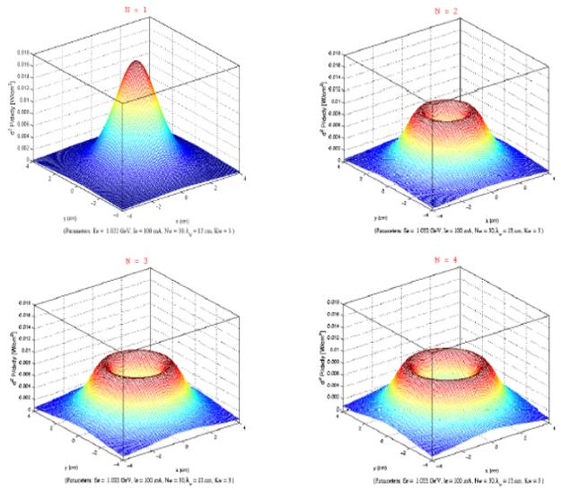
Figure 3: Spatial distribution of 1st, 2nd, 3rd, and 4th harmonic radiation power of a helical wiggler. Parameters for the calculation:  $E_e = 1$  GeV,  $I_e = 100$  mA,  $N_w = 30$ ,  $\lambda_w = 12$  cm,  $K_w = 3$ ; the distance from the wiggler center to the screen is 27 m.
