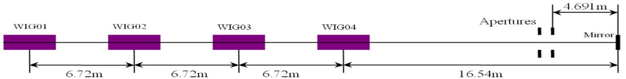
Figure 4: Layout of the OK-5 wigglers in Duke storage ring. Two of them have been installed at the ends of the south straight section of the ring; other two will be installed into the middle of the south straight section.
