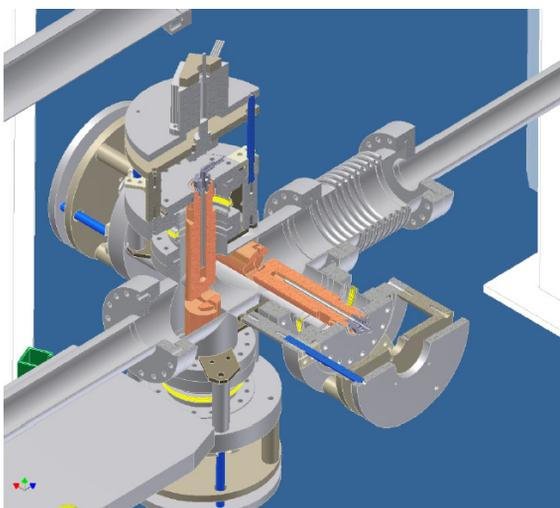
Figure 5: A cut-away view of the water cooled apertures.
