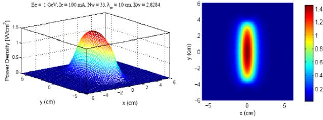
Figure 1: Spatial distribution of planar wiggler radiation power. Parameters for the calculation:  $E_e = 1$  GeV,  $I_e = 100$  mA,  $N_w = 33$ ,  $\lambda_w = 10$  cm,  $K_w = 2.8$ ; the distance from the wiggler center to the screen is 27 m.
