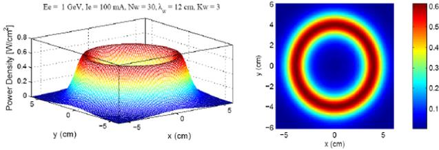
Figure 2: Spatial distribution of helical wiggler radiation power. Parameters for the calculation:  $E_e = 1$  GeV,  $I_e = 100$  mA,  $N_w = 30$ ,  $\lambda_w = 12$  cm,  $K_w = 3$ ; the distance from the wiggler center to the screen is 27 m.
