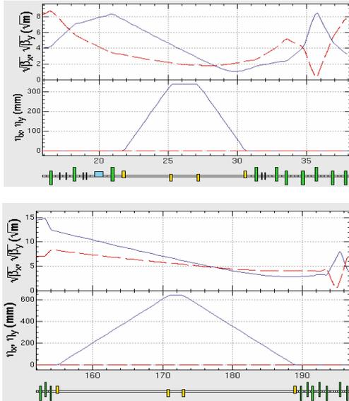
Figure 3: Optics for first (top) bunch compressor and second (bottom) bunch compressor.
