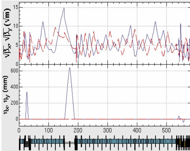
Figure 2: Twiss parameters from injector exit to undulator entrance.
