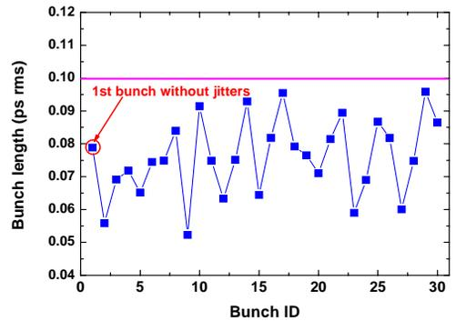
Figure 7: Fluctuation of bunch lengths in the 30 successive bunches under the effects of rf jitters of 0.5 ps rms timing, 0.1 deg. rms phase and 0.05 % rms voltage.
