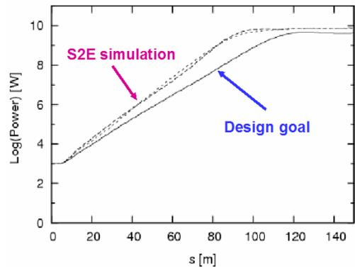
Figure 6: Radiation power as a function of undulator from start-to-end beam simulations.
