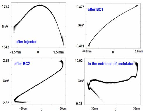
Figure 4: Longitudinal beam distributions from the start-to-end beam simulations.
