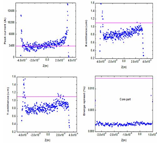
Figure 5: Slice beam distributions in the entrance of the undulator.
