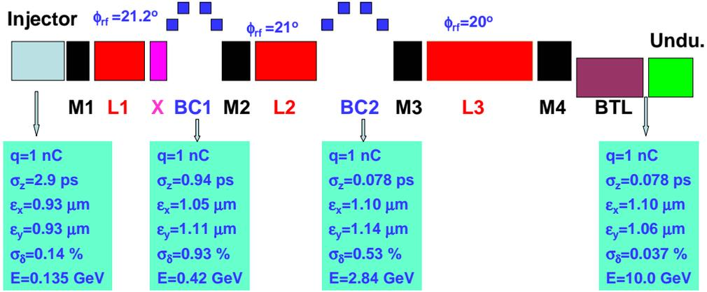
Figure 1: Schematic for a 10.0 GeV FEL facility.
