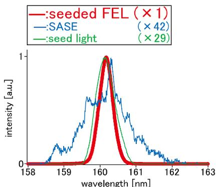
Figure 2: Comparison of spectra between seeded FEL and SASE after one undulator.
