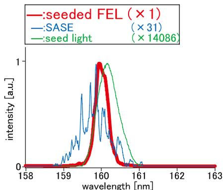
Figure 3: Comparison of spectra between seeded FEL and SASE after two undulators.
