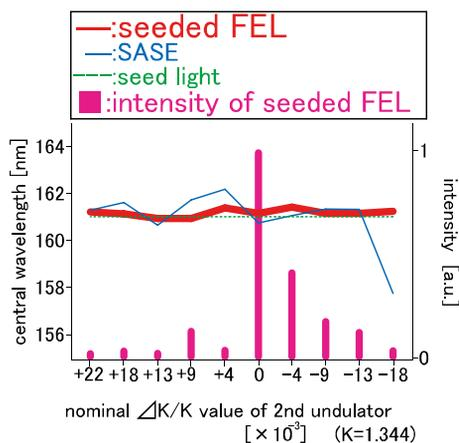
Figure 5: Dependence of lasing wavelength as a function of K value of the second undulator. K value of the first undulator is fixed to 1.386.
