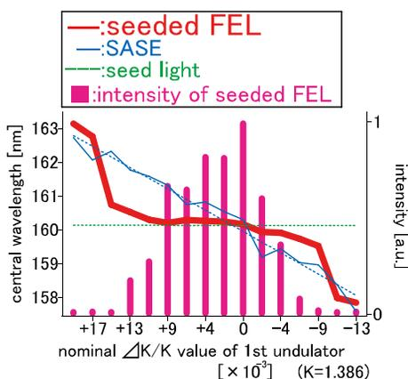
Figure 4: Dependence of the lasing wavelength as a function of K value of the first undulator. The gap of the second undulator is fully opened.
