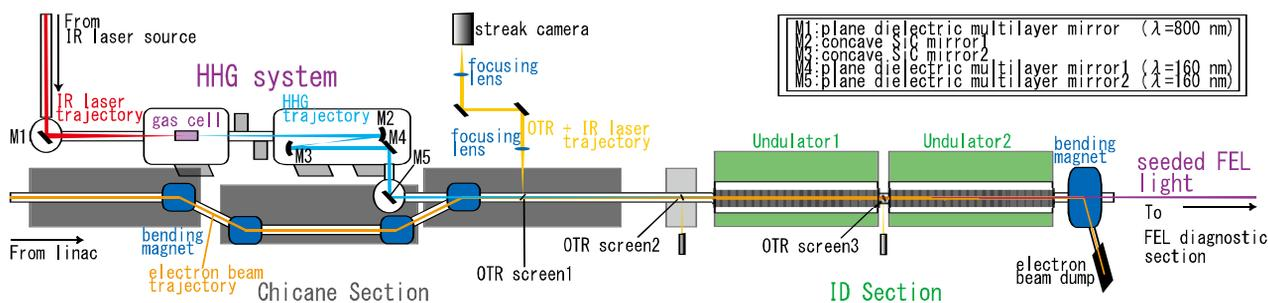
Figure 1: Layout of the seeding FEL at SCSS Test Accelerator.
