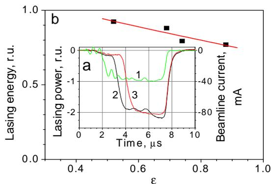
Fig. 6. a. 1- Shape of the macro-pulse current at the FEL undulator entrance (right scale), 2 and 3- Shapes of the
