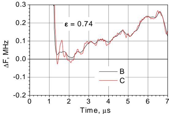
Fig. 3. B: Deviations of the frequency in the microtron accelerating cavity, C: Bunch repetition rate deviations of the extracted current.
