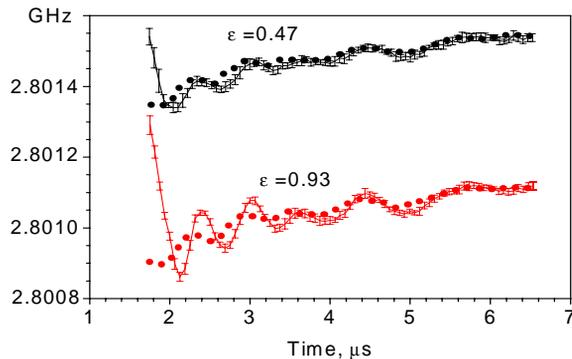
Fig. 5. Measured deviations in the bunch repetition rate, solid line with error bar, and in the magnetron frequency, dots, during the macro-pulse for two values of the detuning parameter.
