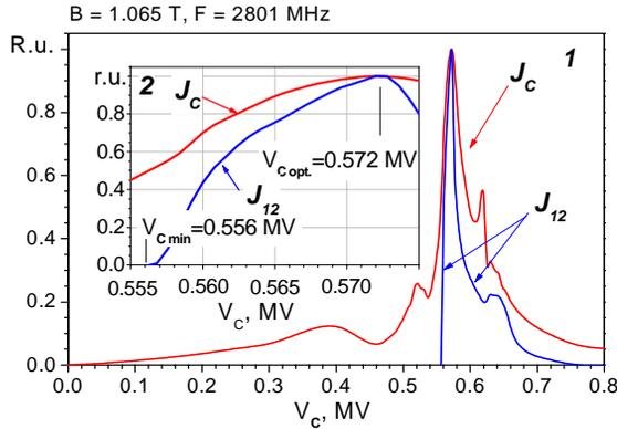
Fig. 1. Normalized amplitudes of the loading current,  $J_C$ , and the accelerated current extracted from the 12-th orbit,  $J_{12}$ , (in relative units) vs. the accelerating cavity voltage. In the inset, (2), the curves  $J_C$  and  $J_{12}$  are plotted in detail in the neighborhood of the microtron operating conditions.
