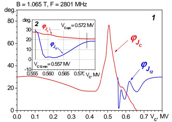
Fig. 2. Phases of the loading current,  $\phi_{J_C}$ , and the extracted current,  $\phi_{J_{12}}$ , as functions of the accelerating cavity voltage  $V_C$ .
