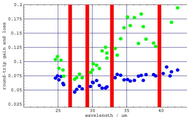
Figure 5: Cavity round-trip loss (blue) and small-signal gain (green) recorded at 40 MeV beam energy. The red stripes denote inaccessible wavelength ranges.
