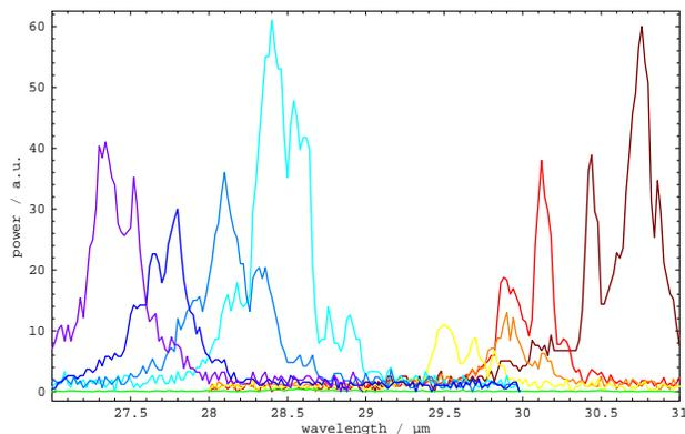
Figure 2: Measured spectra when tuning the wavelength by varying the undulator gap over the spectral gap around 29  $\mu\text{m}$ .
