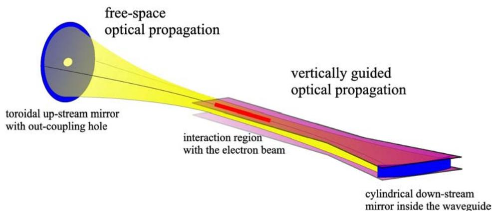
Figure 1: The ELBE-U100 optical resonator is equipped with a waveguide spanning from the undulator entrance to the downstream mirror with free-space optical propagation to the upstream mirror.
