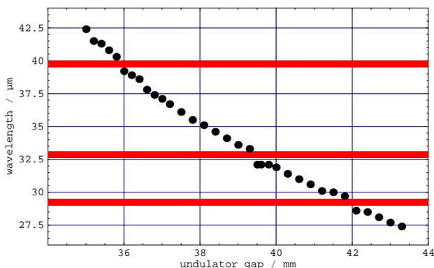
Figure 3: Wavelength versus undulator gap measured at 40 MeV electron beam energy. Even though the lasers are working for almost all settings of the undulator gap, some wavelengths are inaccessible (like 29  $\mu\text{m}$  or 33  $\mu\text{m}$ ) which are shown with red stripes.
