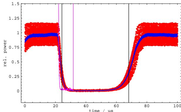
Figure 4: Measurement data for determination of the round-trip gain and cavity losses.
