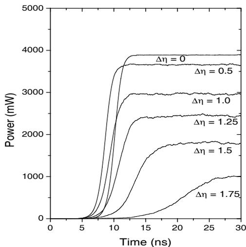
Figure 4: Evolution of power in the surface mode in SP-BWO for different values of  $\Delta\eta$  as calculated by numerical simulation. Beam current is taken to be 45 mA. Other parameters used in the numerical simulation are described in the text.
