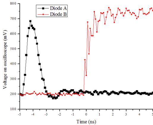
Figure 5. Photo diode signals while hit by electrons directly. Arrival information is between 200 and 500 ps. (The different shape of the signal is due to different termination of the signals).
