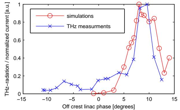
Figure 4. The THz signal intensity as a function of linac phase (providing the energy chirp for compression).
