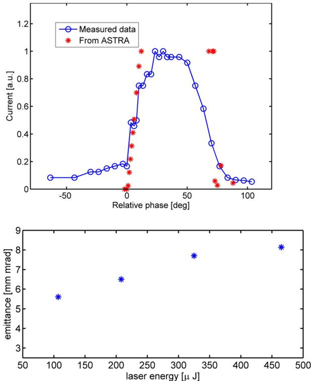
Figure 3. RF gun performance. (a) Current output from the gun at different RF phases (circles-measurement, stars-simulation). (b) Emittance as a function of laser energy (charge significantly below 0.5 nC).
