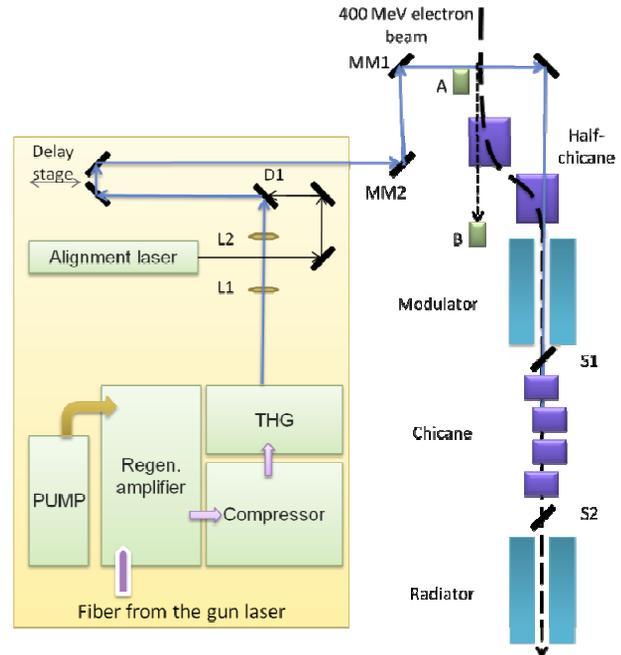
Figure 2. Seed laser layout and optics to focus the laser beam into the modulator. L1 and L2 are lenses for focusing of the laser beam inside modulator. MM1 and MM2 are remote controlled mirrors. S1 and S2 are screens used for alignment. A and B are diodes used for time synchronization.
