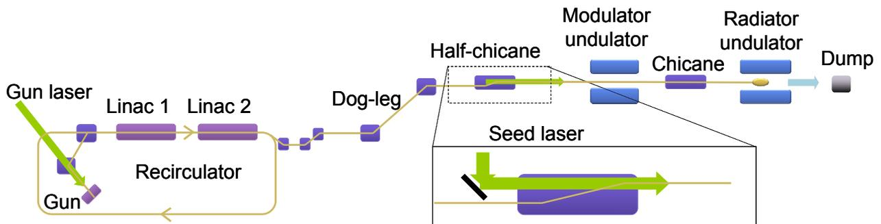
Figure 1. Layout of the MAX-lab test-FEL.
