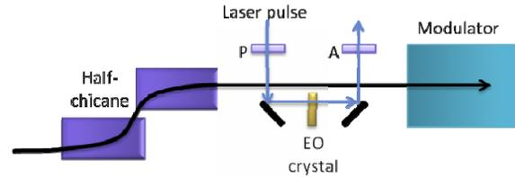
Figure 7. Schematics of the planned electro-optical technique to synchronize the seed laser pulse and electron bunch more precisely.
