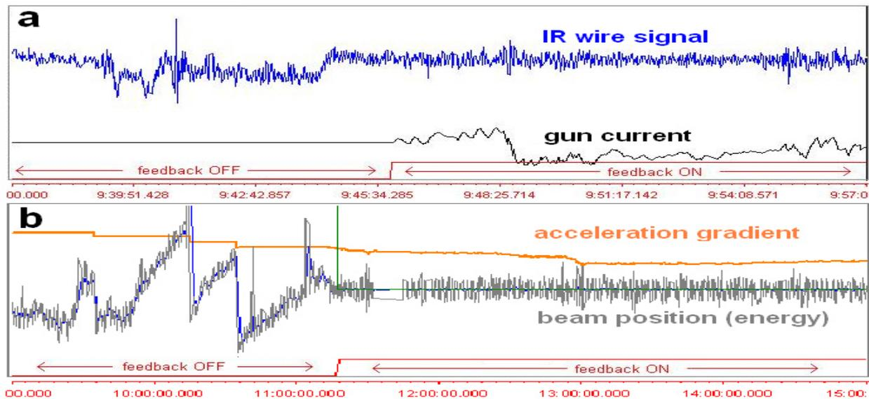
Figure 8: Effect of feedback control for FEL power (a) and FEL wavelength (electron beam energy) (b).
