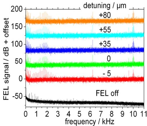
Figure 3: FEL power fluctuation spectra of U100 FEL at different detuning (0-11 kHz).
