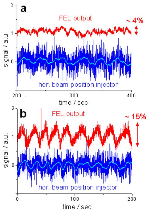
Figure 2: Low-frequency FEL power modulation in correlation with the horizontal injector beam position. a: At small FEL detuning (10  $\mu\text{m}$ ), b: At maximum FEL detuning (80  $\mu\text{m}$ ).
