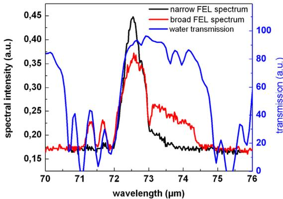
Figure 1: Spectral FEL pulse modification by water absorption windows.
