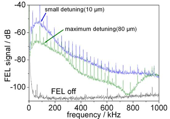
Figure 4: FEL power fluctuation spectra of U100 FEL at different detuning (0-1 MHz).
