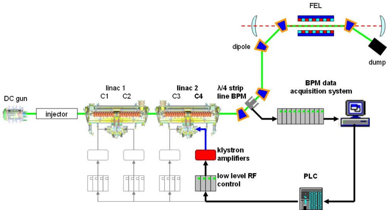
Figure 7: Feed-back system for energy (FEL wavelength) stabilization.
