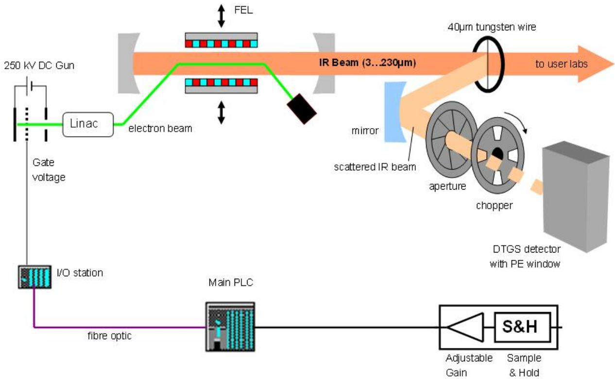
Figure 6: Feed-back system for FEL beam power stabilization.
