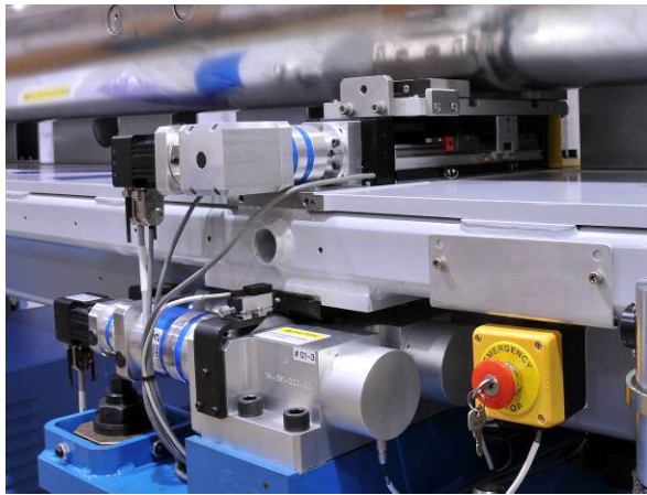
Figure 5: The undulator is mounted on a translation slide that is attached to the girder. The double CSM is shown below the girder, mounted on the intermediate plate.
