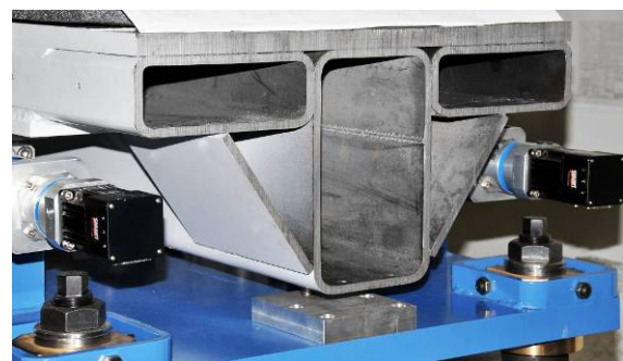
Figure 4: A cross section of the support girder mounted on the intermediate plate.
