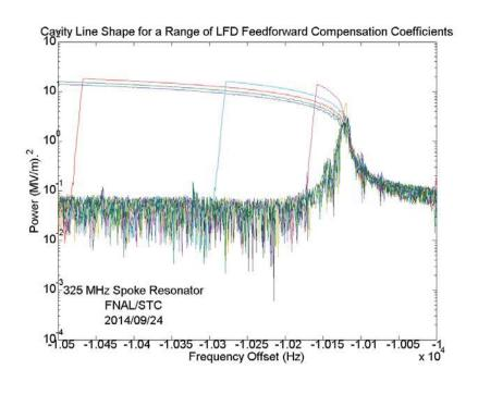
The LFD feedforward coefficient was calculated several ways, including fitting detuning during cavity decays.
