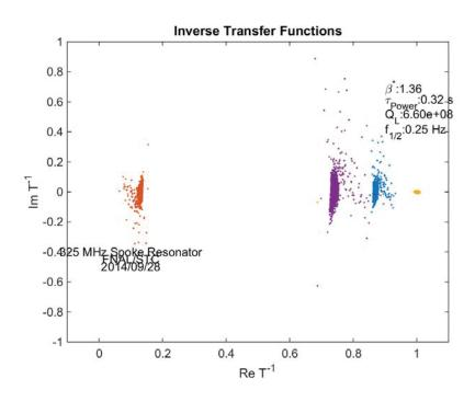
Step one was calibrating the cavity coupling. Loaded Q (and thus bandwidth) was calculated from the cavity decay time.
