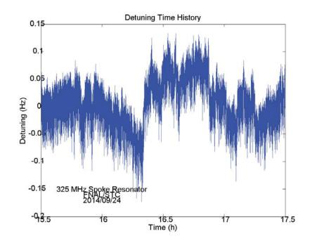
Initial efforts at direct piezo feedback of microphonics induced detuning showed good promise, but exhibited a long timescale drift. A slow compensation loop was added in the Matlab controller to help correct for this very slow drift.
