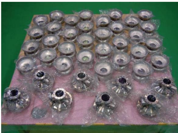
① 4 sets of 9-cell cavity parts
