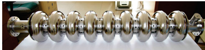
PKU No.04(Large Grain: TESLA Shape) 2nd. Vertical Test 04/25/2013 Local Grinding, EP-II(20μm), Water flow(1.5hrs), FM_20_2%(50C,60min), H.P.R.(~7hrs), Baking(140C, 44hrs)
