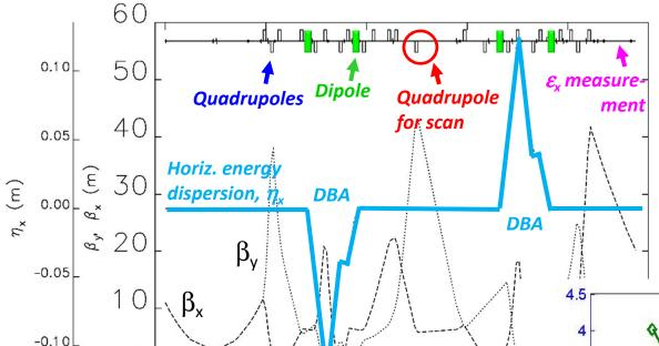
Quadrupoles ensure  $\pi$ -phase advance between dipoles and proper values of  $\beta_x$ ,  $\alpha_x$  to cancel the CSR-emittance.
