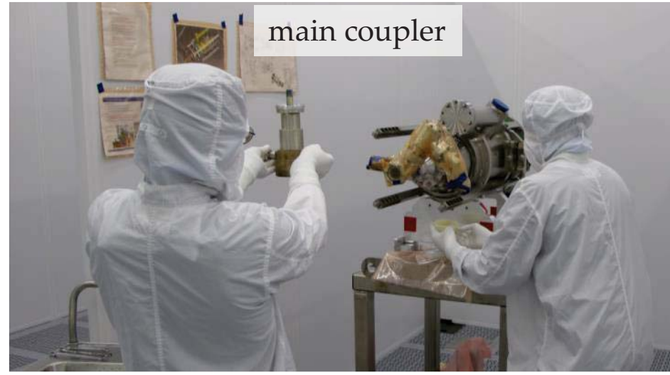
successfully leak checked
