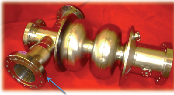
Large coupling port for modified KEK high-power couplers
