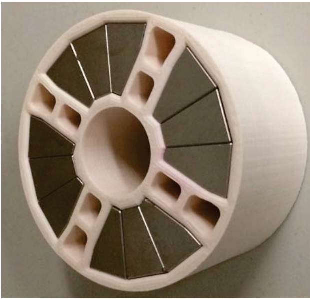
Figure 5: A picture of the modified Halbach quadrupole. The housing of the permanent magnet wedges is made by a 3D printer.
