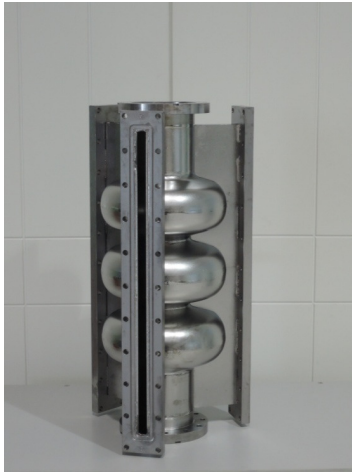
Figure 4: 1.3GHz 3-cell slotted cavity.
