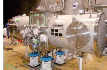
Figure 3: Main accelerator module of cERL in KEK.
