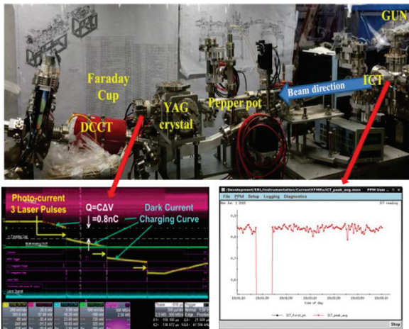
Figure 7: Straight beam line with beam diagnostics components (top). Dark current (slop) and photocurrent (spikes) measured one faraday cup (left bottom). Cross calibration charge measurements at ICT (right bottom).
