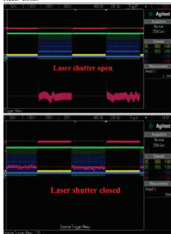
Figure 5: Faraday cup (1M \Omega termination) signal during first beam test of ERL 704 MHz SRF Gun. Top: laser shutter open 1.09V; bottom: laser shutter closed 38mV. It corresponds to dark current 38nA, photocurrent 1.09 mA.
