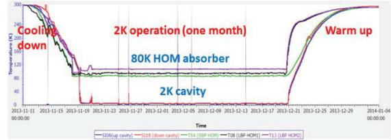
Figure 5: Example of cryogenic operation for the run at December of 2013. Temperatures of cavities are shown by red and blue lines.
