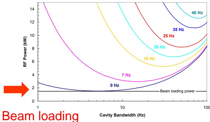
RF power versus cavity bandwidth for different microphics levels at a system with 1.5 kW beam loading
