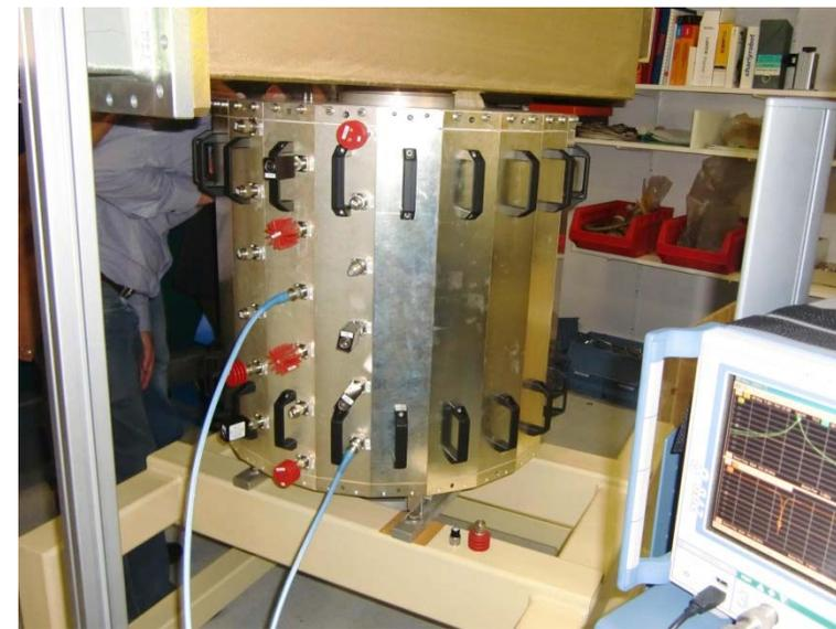
Prototyp of a cavity combiner
