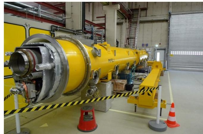
Cryomodule for Euro-XFEL
