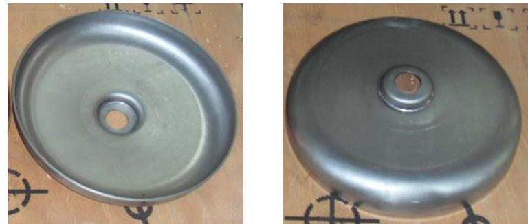
$\beta=0.45$ , 650 MHz cavity half cells
