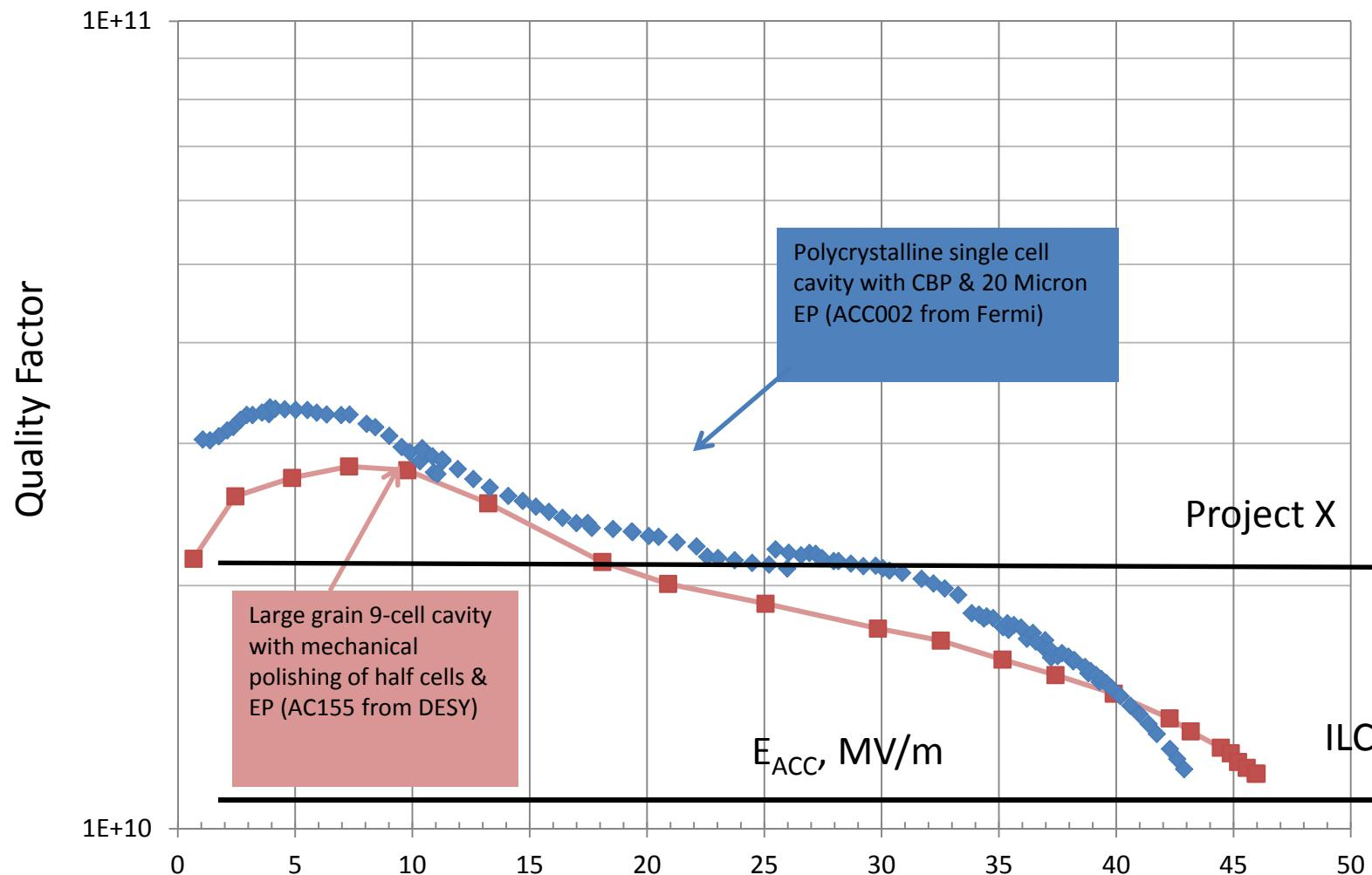
Recent high Q results on Tesla-Type cavities. Do grain boundaries have a negative effect on Q(Low, Mid, and High)?
