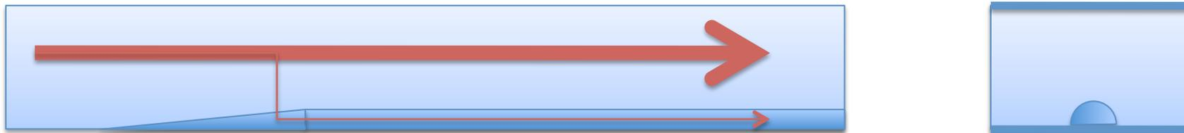
When  $v_t < v_{critical}$  (some critical value), almost RF waves travel outside of the dielectric material.
