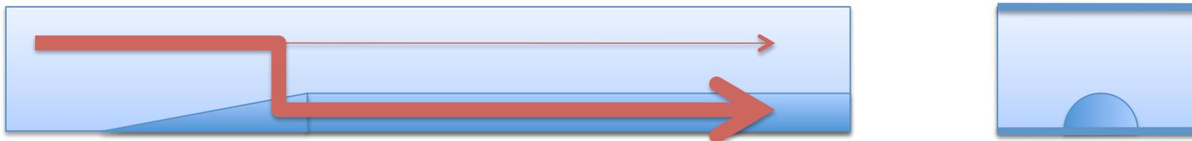
When  $v_t > v_{critical}$  (some critical value), almost RF waves travel in the dielectric material.
