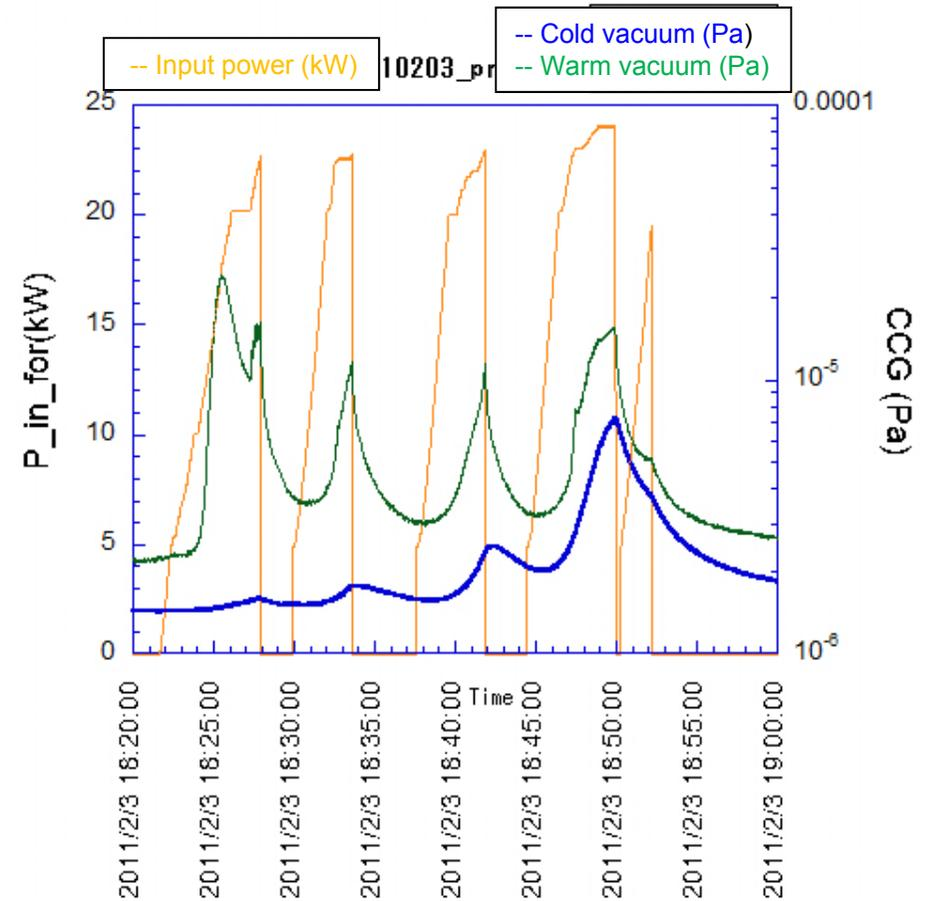
After warming up and exposing to air for 4 hours, the coupler was cooled down to Liq. N<sub>2</sub> temperature again and we fed the power. We can feed the power up to 24kW smoothly. **Processing effects could keep the coupler.**
