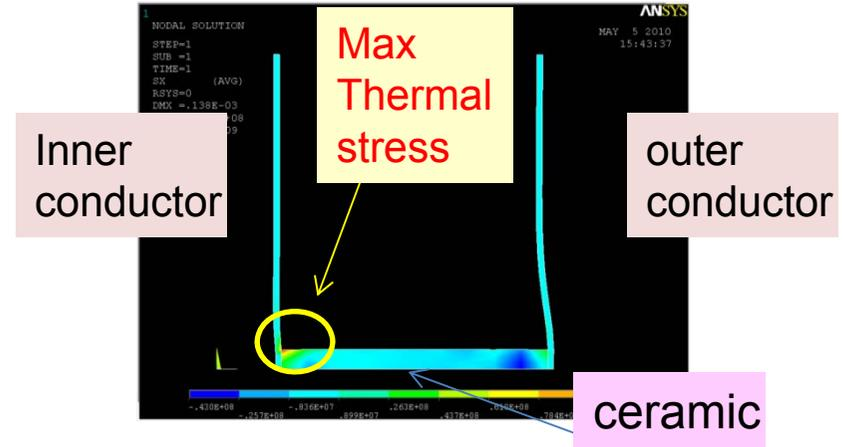
After 5<sup>th</sup> thermal cycle test between 80K and 300K, old ceramic was broken
