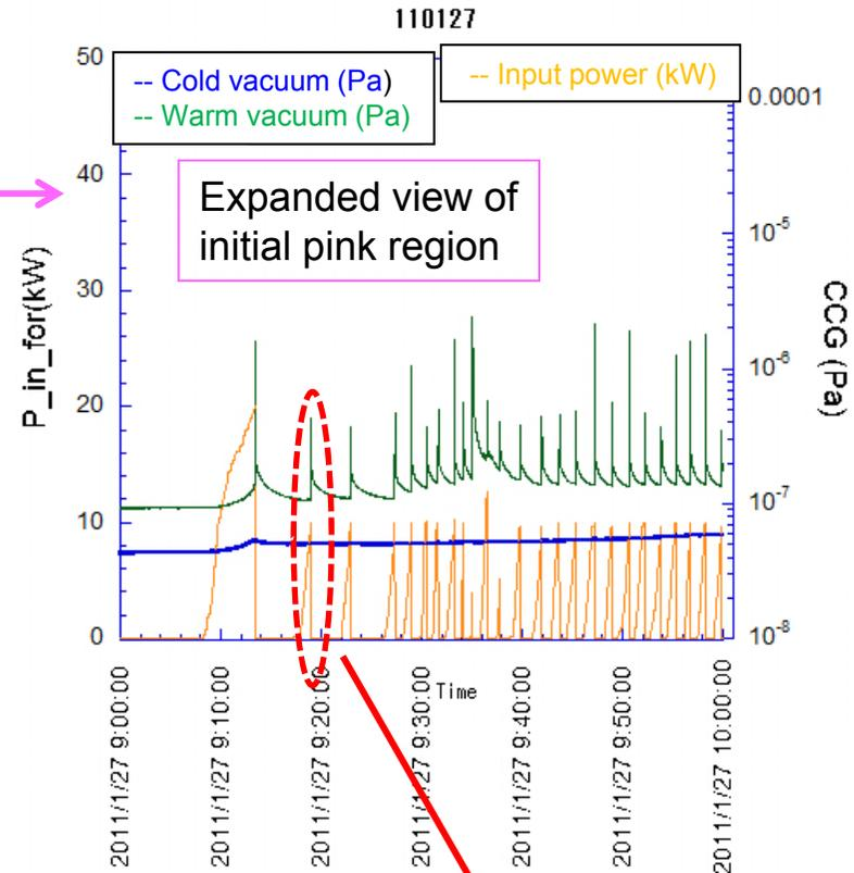
At 20kW, suddenly arc (arc2) and vacuum (CCG2) interlocks worked. feeding power could not overcome 10kW level under CW power feeding.
