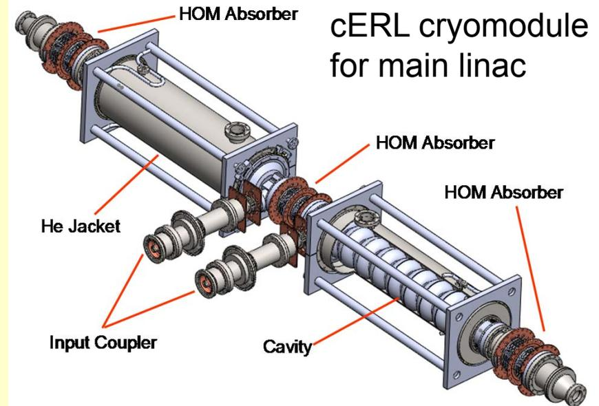
cERL cryomodule for main linac
