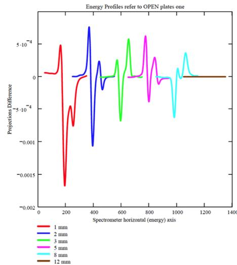
With closed gap the distribution is close to that from the HE slit - opening gap increases the distortions
