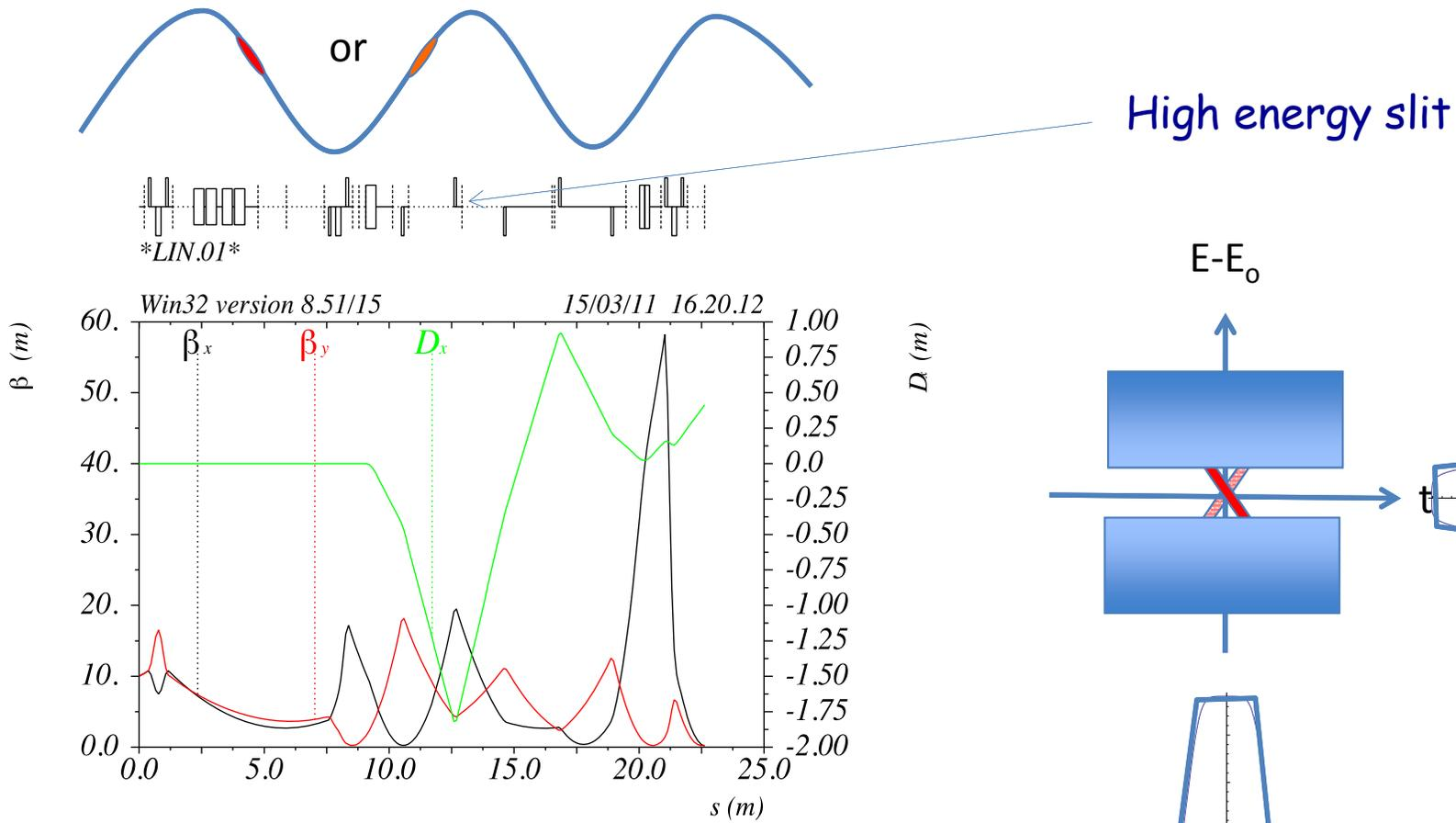
Optical function of the transport line from linac exit to spectrometer beam profile monitor. Energy collimator is located at position of 12.5m and magnet with shielding plates is installed at 20m position
