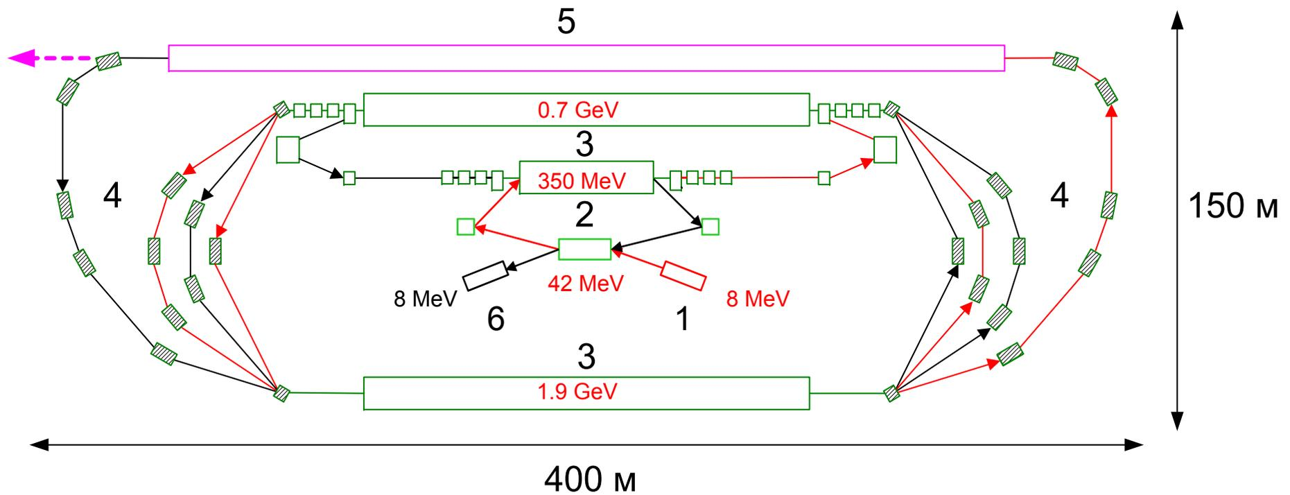
1 – injector, 2 – preliminary accelerating system, 3 – main accelerating RF structure, 4 – magnets, 5 – undulator, 6 – dump.
